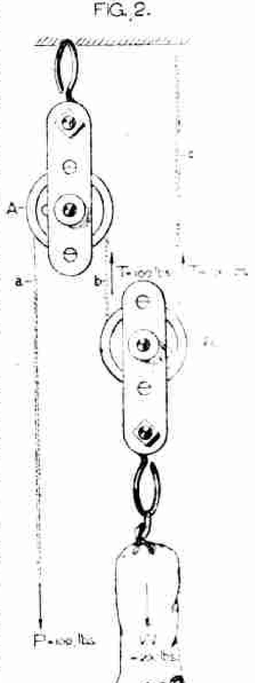
he previously raised 100lbs. The explanation is simple. There are two distinct parts in the cord "b" and "c," by which the load is suspended, and the strain on each part must be the same, 100lbs. Now the strain on the two parts of the rope, "a" and "b," passing over the fixed pulley "A" is the same in each case as before—that is, 100lbs., so that the man pulling must only be exerting a force of 100lbs. to lift 200lbs.
