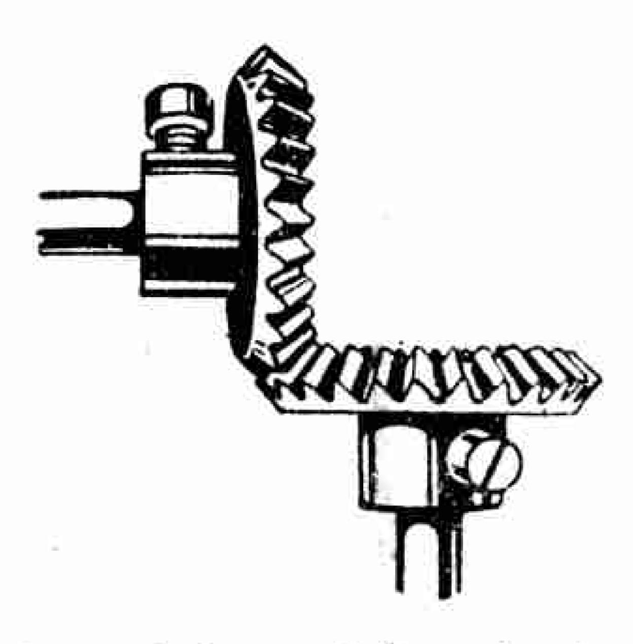
Rods or shafts at right angles have previously been connected in the Meccano system by contrate wheels and pinions, but the bevel gears are much superior and are based on proper engineering practice. There is less friction in the bevels than with the contrate wheel and pinion, and further the bevels do not require such accurate setting.
