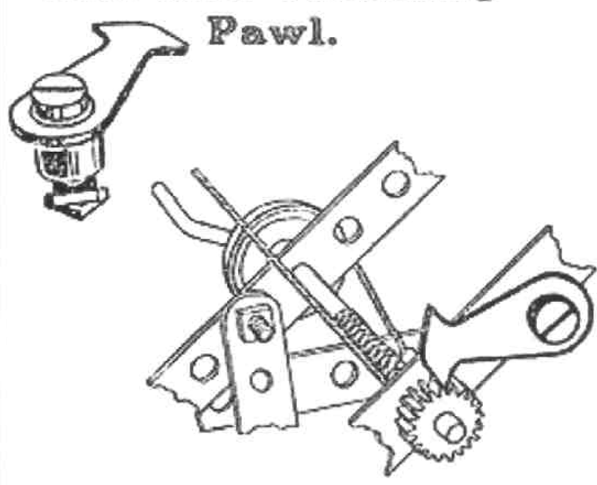
The above is an illustration of the new Meccano Pawl, and an example of its use. This replaces the present pawl, No. 33. It is shown connected to the side strip of a Crano to hold the load while suspended in the air. This pawl moves freely on a pivot bolt secured by lock nutting to the side strip.
