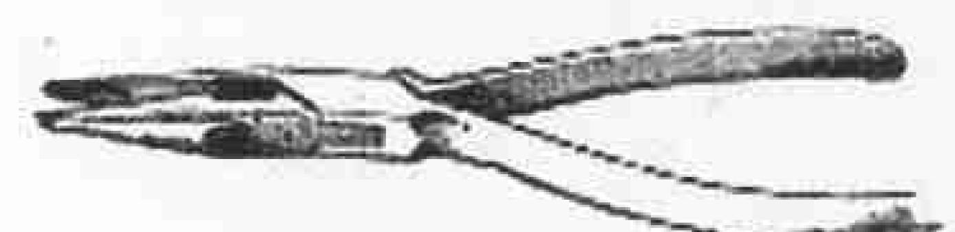
We have often been asked by boys to suggest the best-method of joining or separating the Meccano Sprocket Chain, and for their benefit we are illustrating the best type of pliers to use for this work. No difficulty should be experienced if these sharp pointed pliers are used, and they may be obtained at any good ironmonger's establishment.
