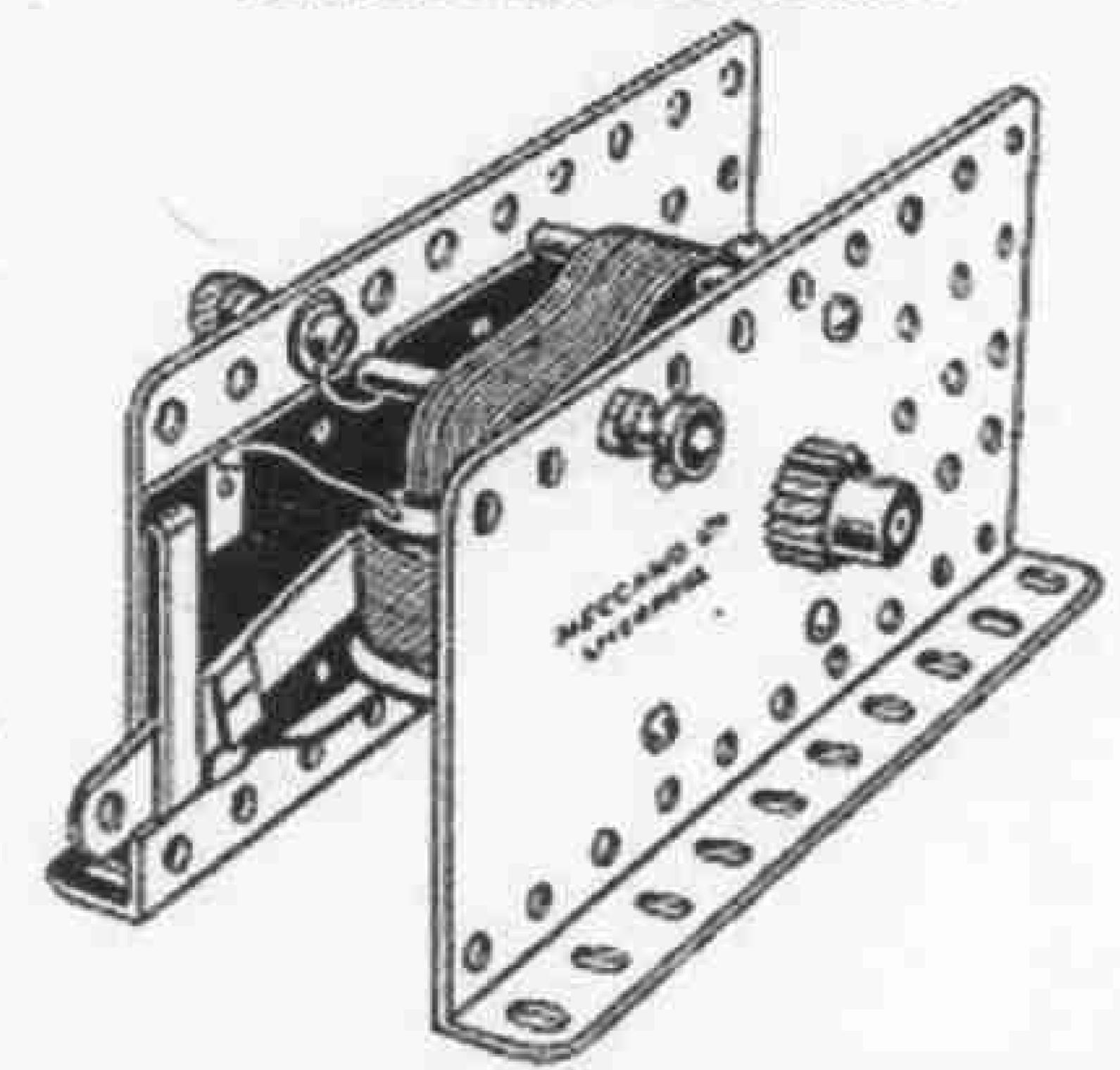
The Meccano Electric Motor has been re-designed, and several new and useful features have been added. It takes 4 volts, and it may be operated by accumulators, dry batteries, or direct from town supply if a suitable transformer is used.
