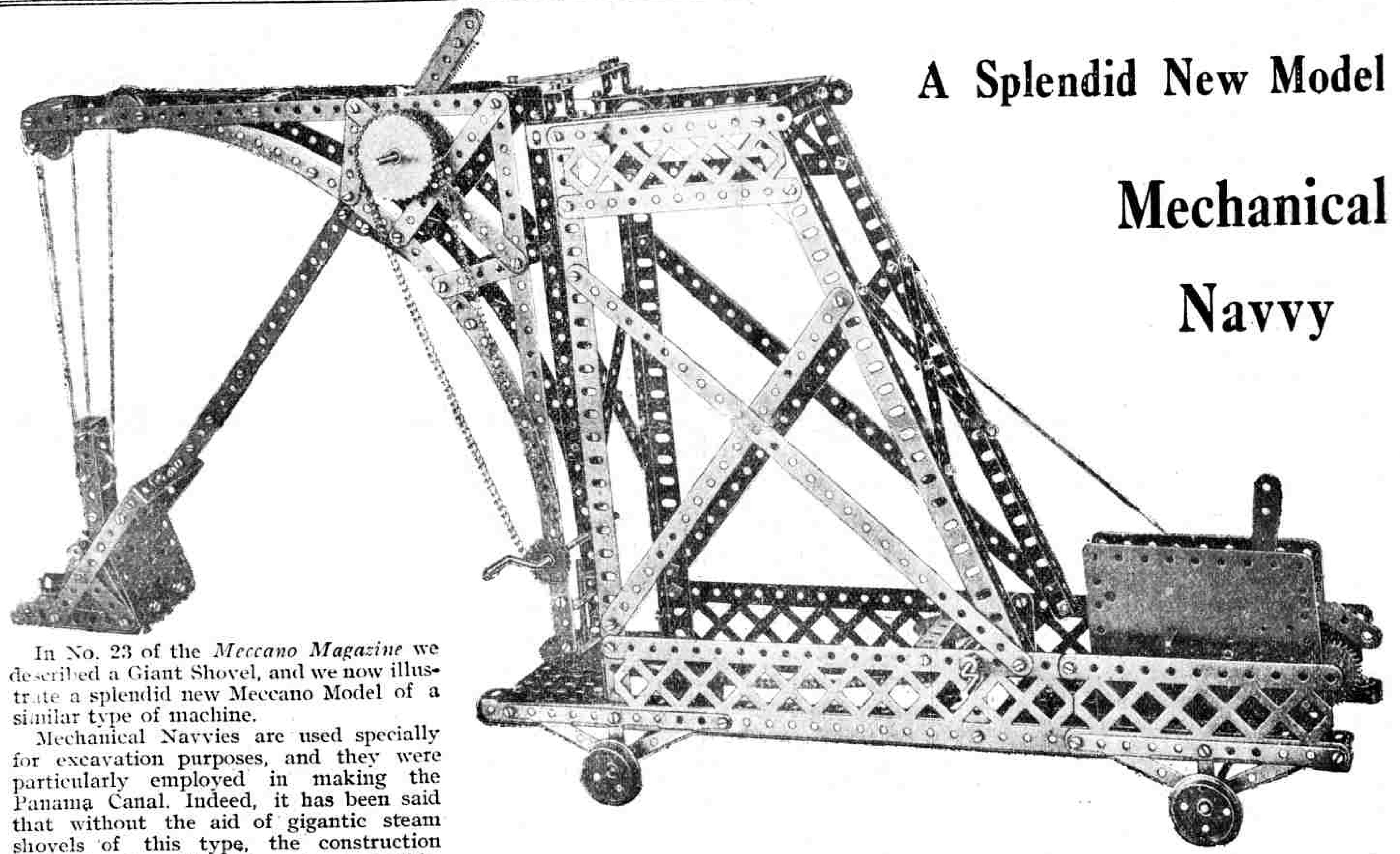
As our illustration shows, the hoisting of the bucket is effected by a Meccano Clockwork Motor, while a hand-operated crank handle actuates the gearing that in actual practice causes the bucket to dig into the embankment that is being removed. Some of these shovels scoop up as much as 12 tons of earth at one bite, and in an eight-hour day will excavate some 4,500 tons of earth, thus marking a great advance over the old methods of spade and pick.
