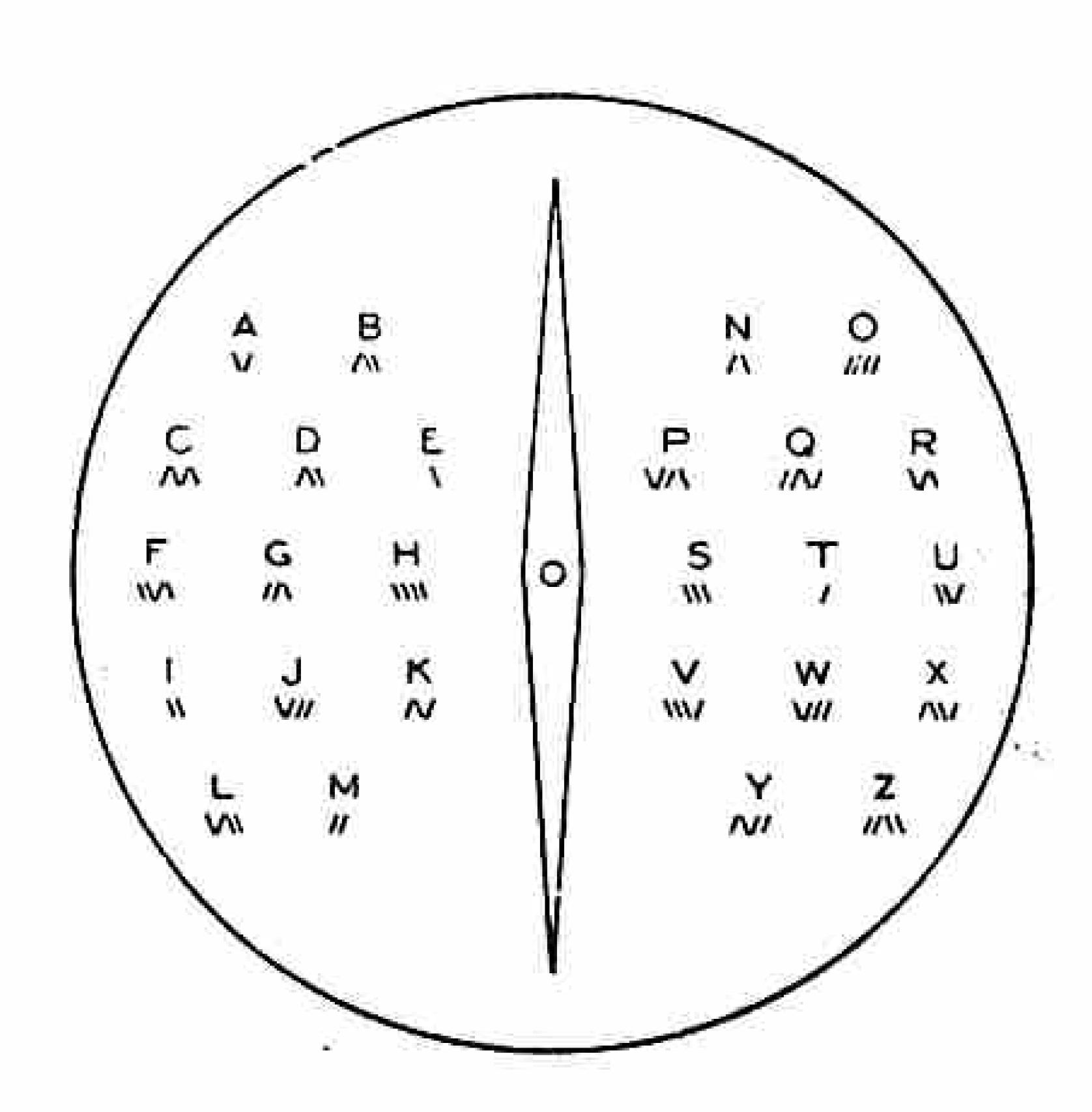
In the second, or "needle" type, a metal needle, pivoted in the centre, is made to deflect to the left or right. On each side of it is fixed a piece of metal with different tones. The ear of the receiving operator is trained to detect the dissimilar notes, caused by the needle being deflected and striking either of the pieces of metal. These sounds represent either dots or dashes.
