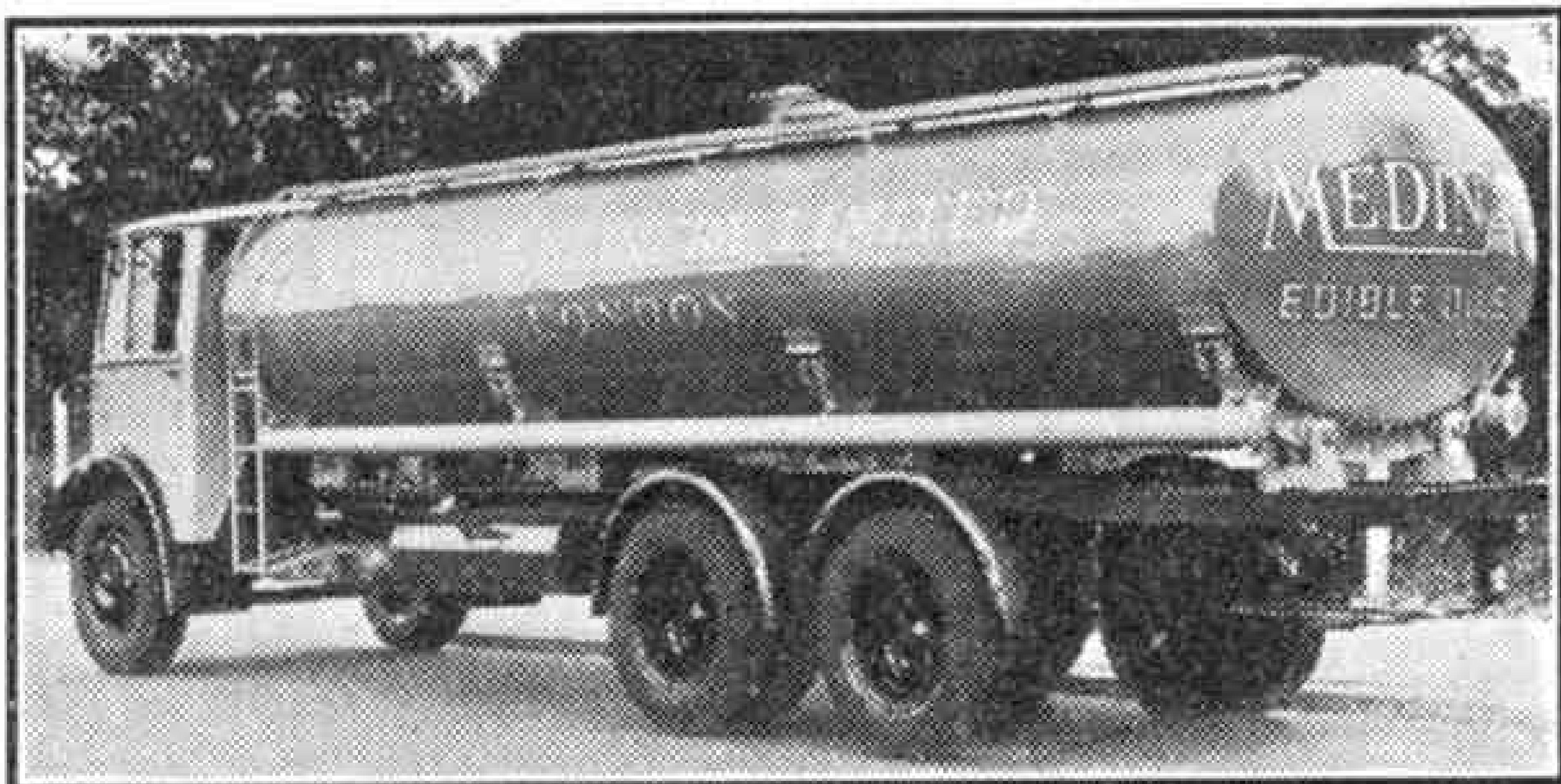
3,500 gall. Aluminium Tank for Vegetable Oil. The illustrations to this article are by courtesy of The Aluminium Plant and Vessel Co. Ltd.
