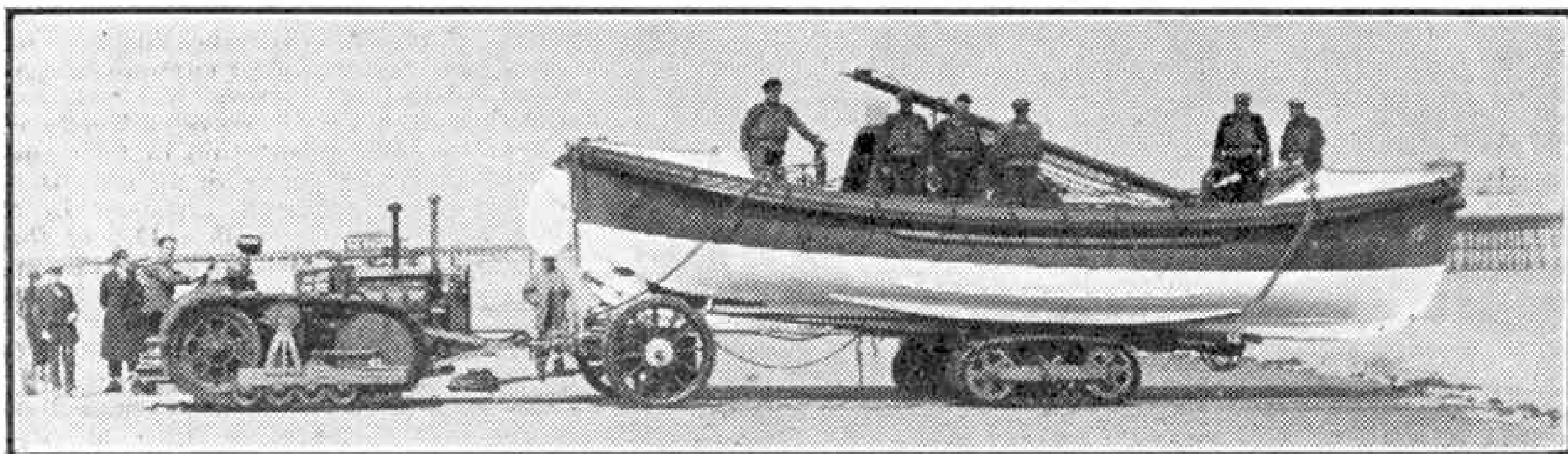
How Orolo girder track units have solved the problem of carrying a life-boat and its carriage over soft beaches, in which ordinary wheels would sink. Photograph by courtesy of Roadless Traction Ltd.
