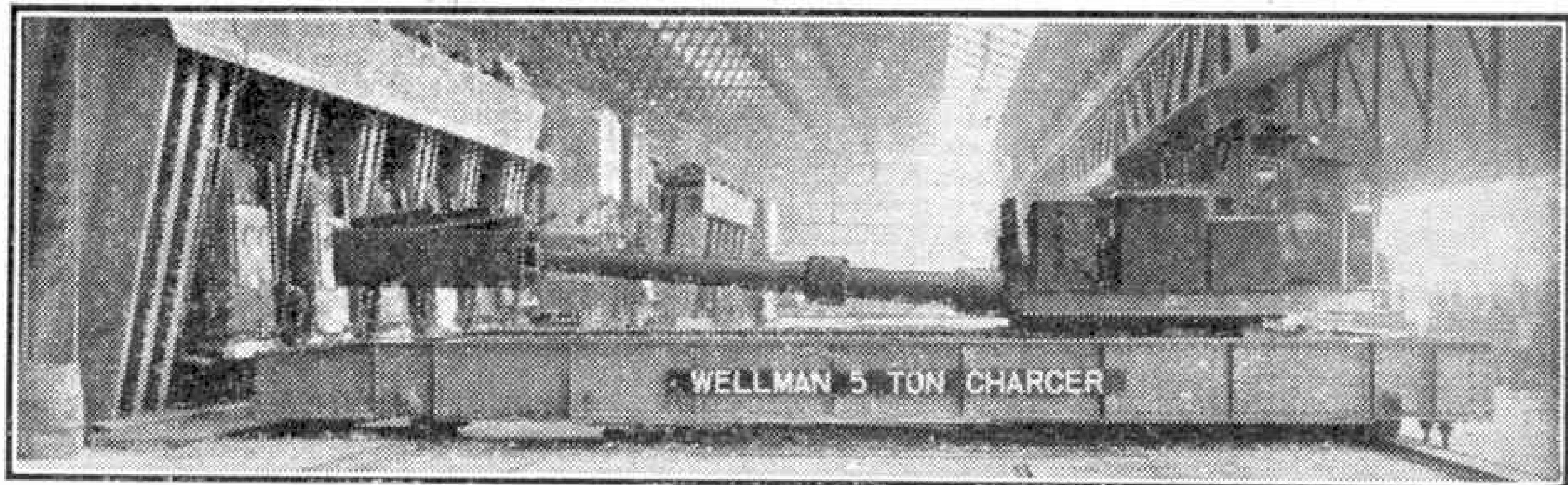
Fig. 3. 5-ton Revolving Low Ground Open Hearth Charging Machine serving Tilting Furnaces.
