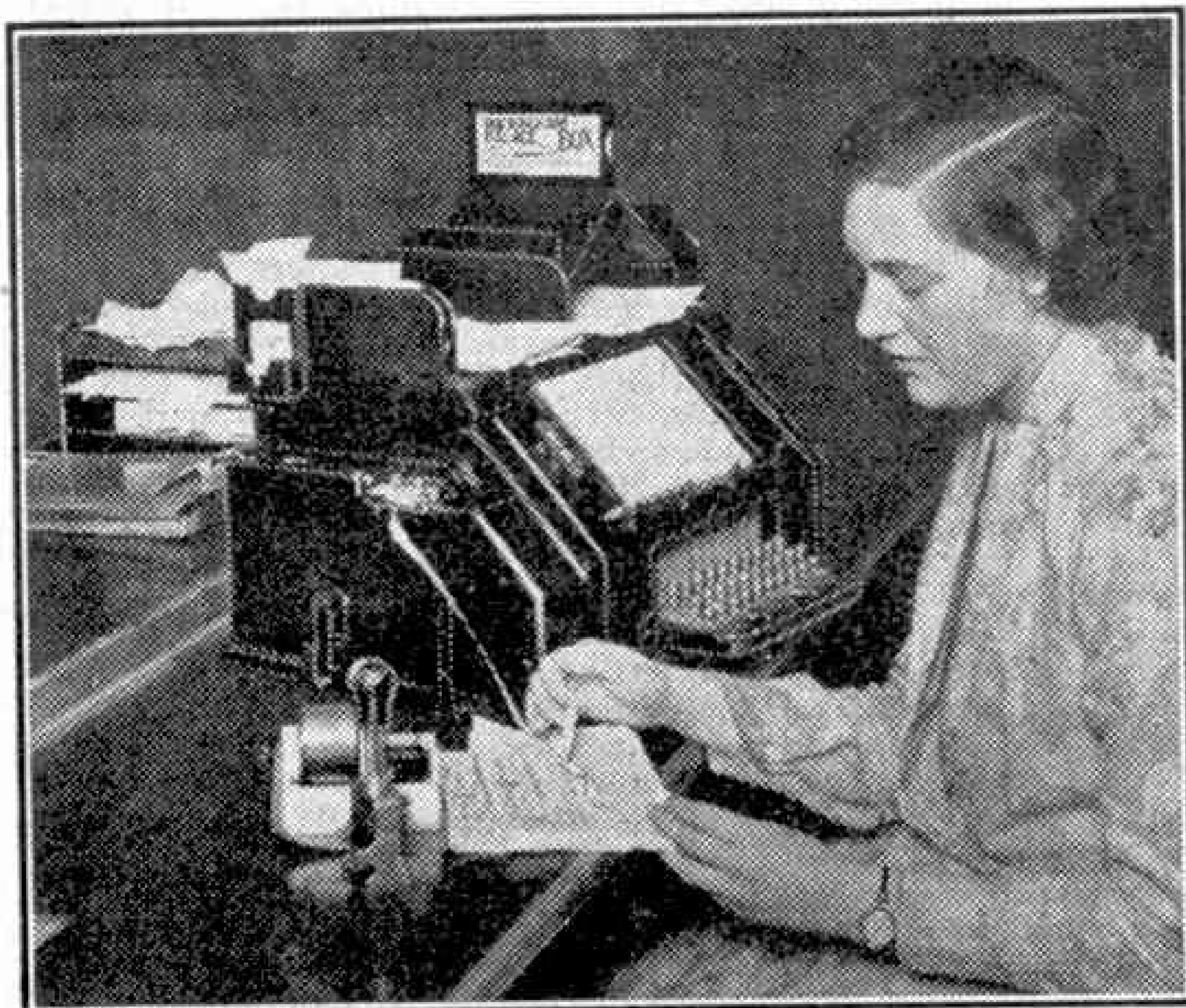
A teleprinter operator pasting typed tape from her machine on a form.
