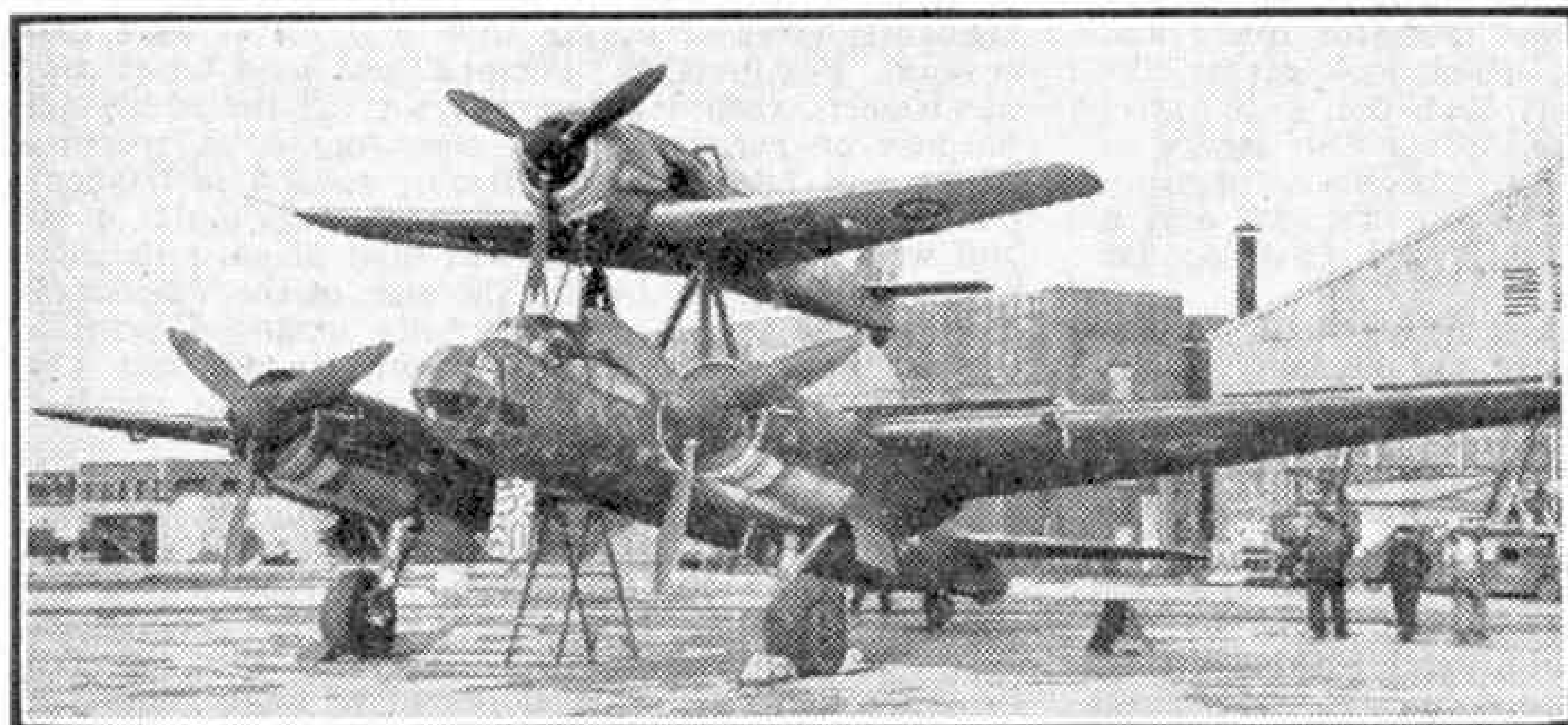
The "Mistel" Composite bomber. Usually the lower component was a Junkers Ju.88 minus equipment and loaded with explosive in the nose, and the upper component was a standard Focke-Wulf 190 fighter. Photograph "The Aeroplane" Copyright.
