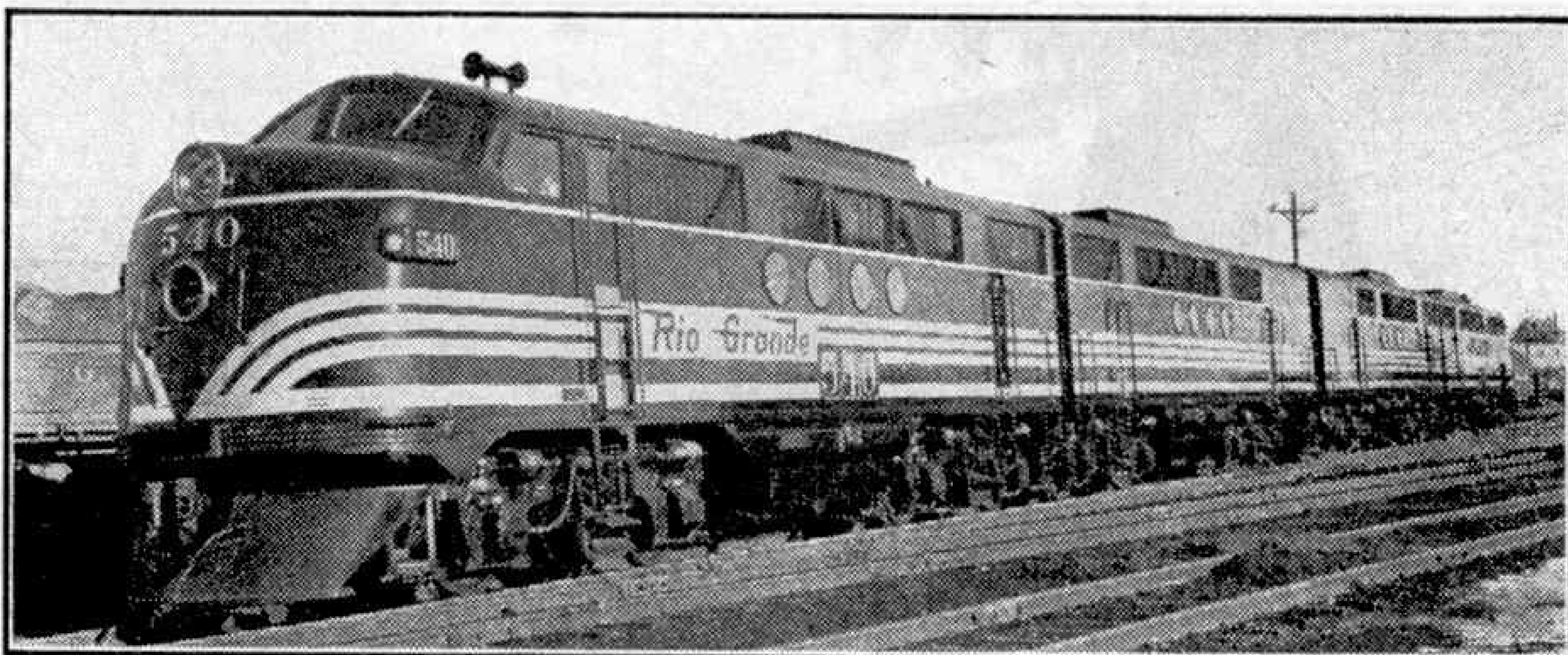
The shape of things to come in Britain? Denver and Rio Grande Western Railroad 5,400 h.p. 4-unit Diesel electric locomotive. Photograph by courtesy of the Denver and Rio Grande Western Railroad.
