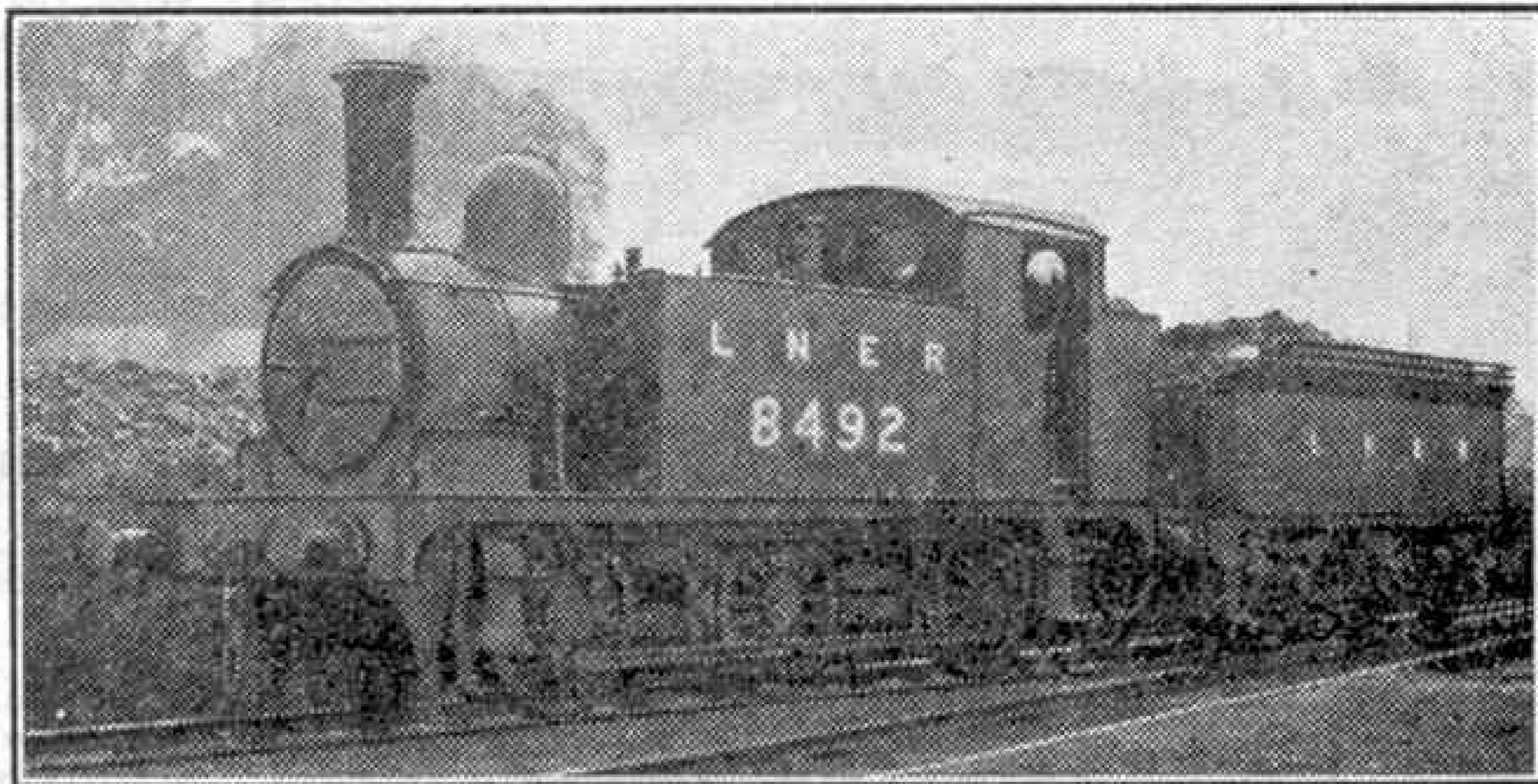
L.N.E.R. No. 8492, of Class J67, fitted with J36 six-wheeled tender for water supply, as used on the Oxton and Lauder branch of the Waverley route. Photograph by courtesy of the L.N.E.R.
