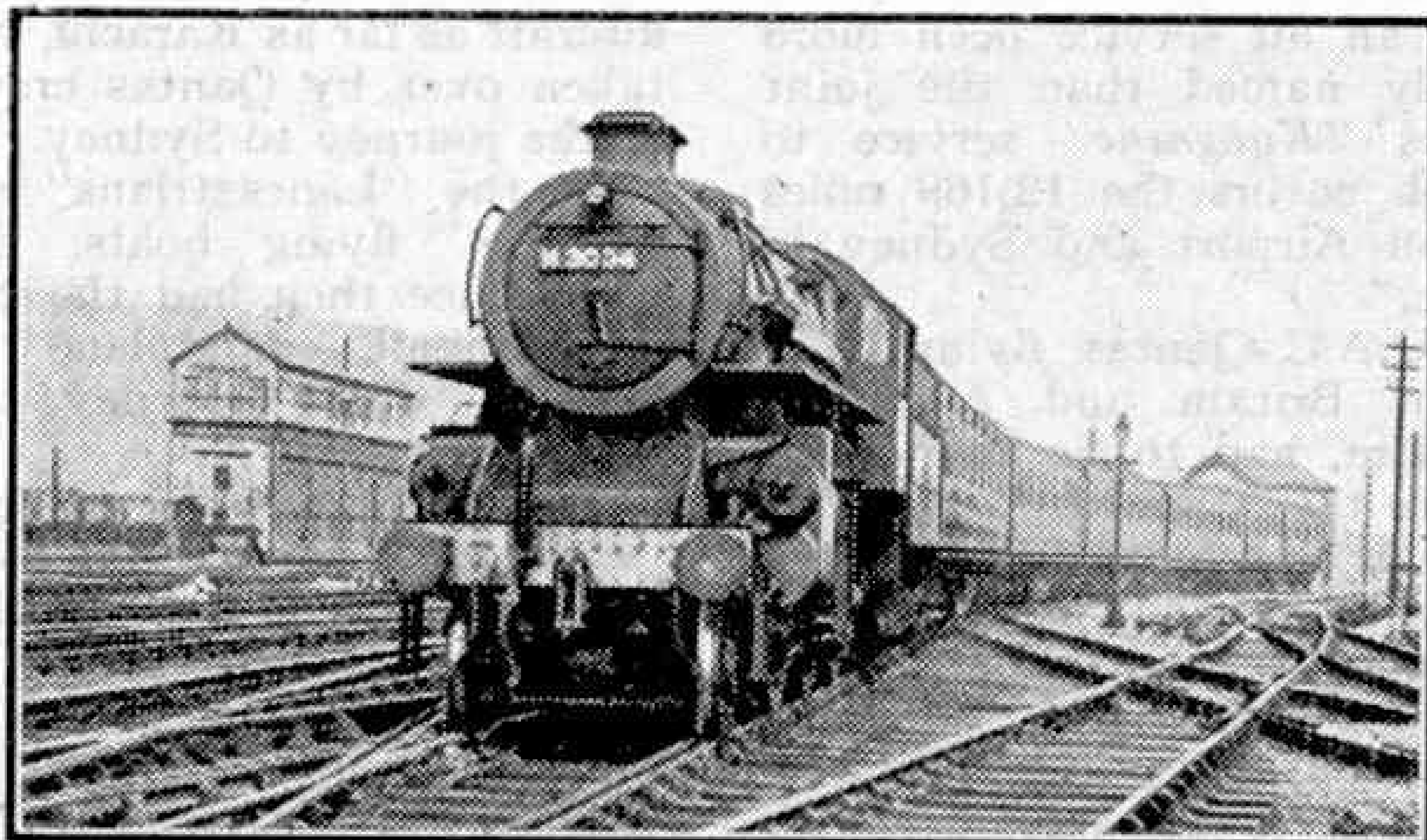
Cambridge - Oxford train entering Bletchley. The engine is London Midland 2-6-0 of Class "4," temporarily numbered M3004. Photograph by H. C. Casserley.
