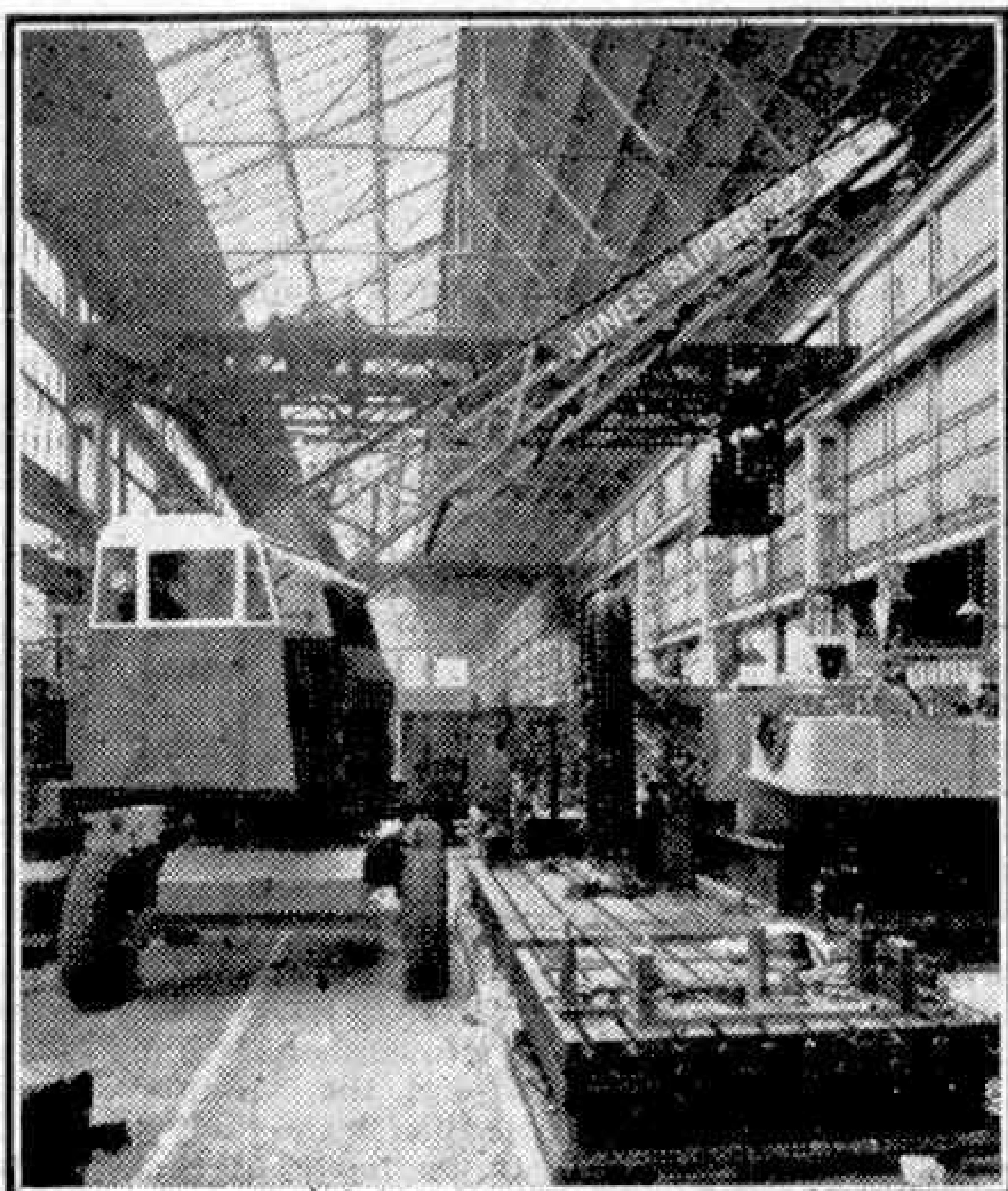
The Jones "Super 22" mobile crane at work in the aisle of a machine shop.
