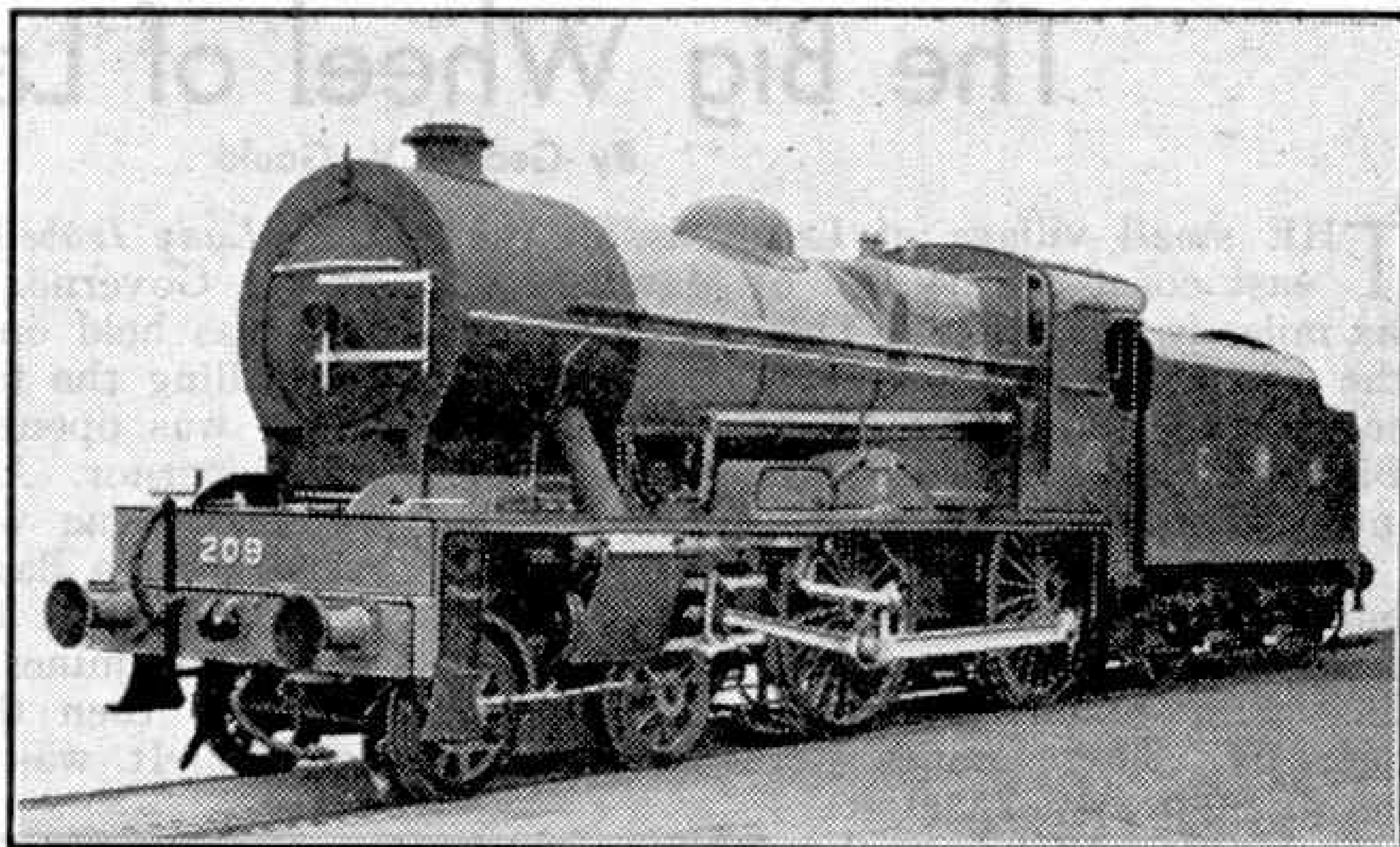
G.N.R.(I) No. 209 "Foyle" of the new 3-cylinder 4-4-0 class referred to on this page. Photograph and details are by courtesy of the G.N.R.(I).
