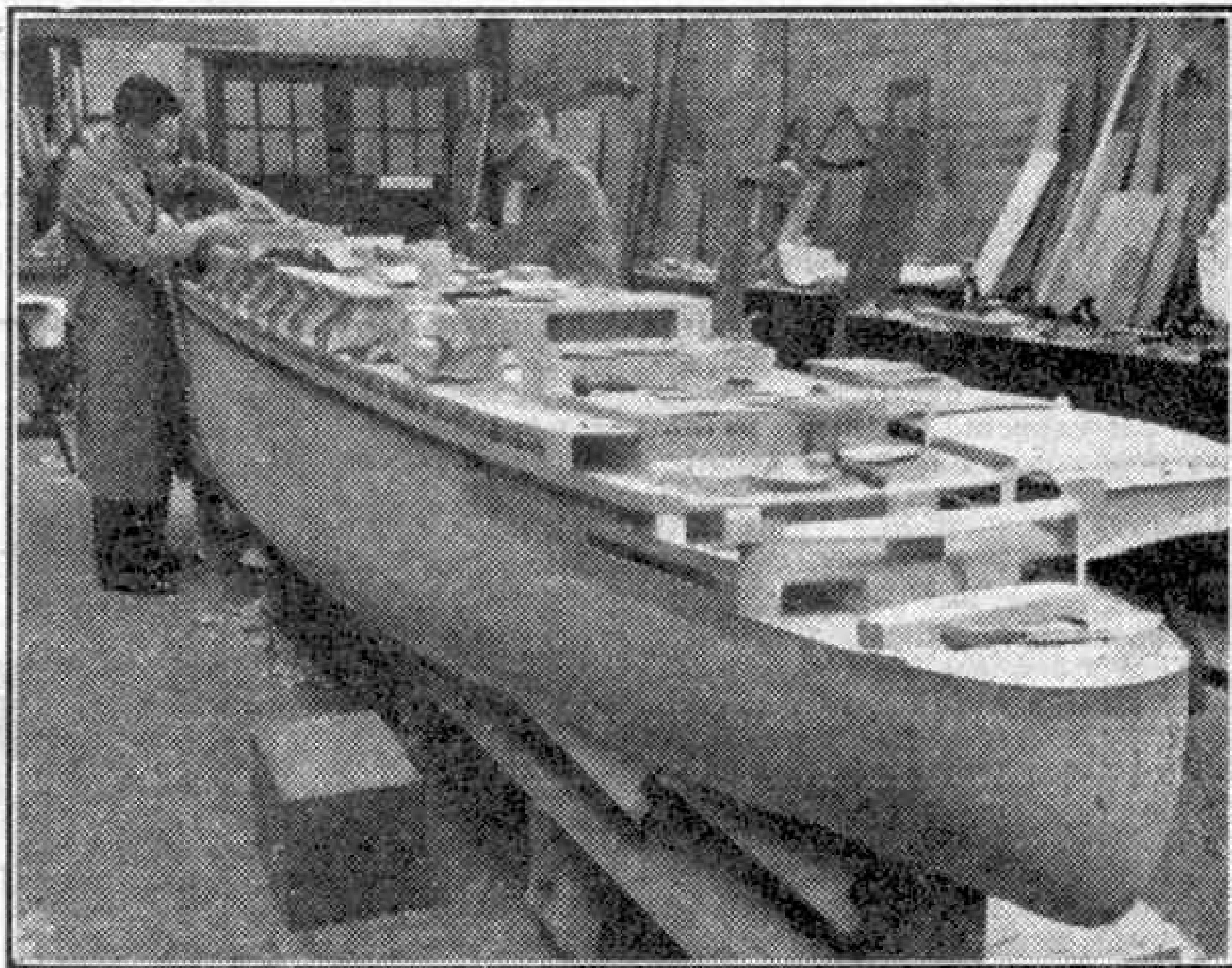
At work on the model of the " Queen Elizabeth ." The hull is complete and craftsmen begin to build up the superstructure on the liner's decks.
