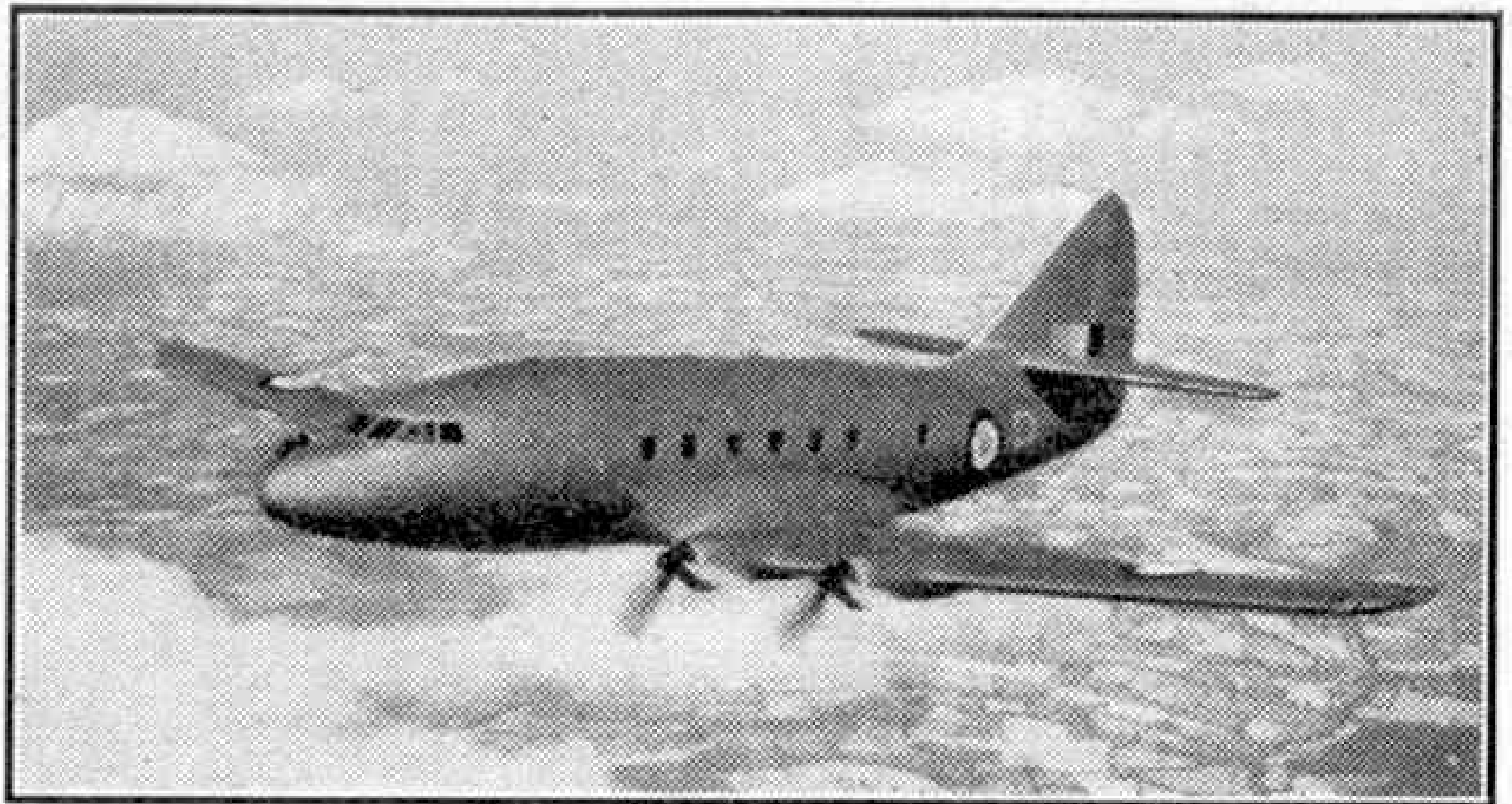
A new photograph of the Armstrong Whitworth "Apollo" air liner, which is powered by four Armstrong-Siddeley "Mamba" propjet engines. Photograph by courtesy of Sir W. G. Armstrong Whitworth Ltd.
