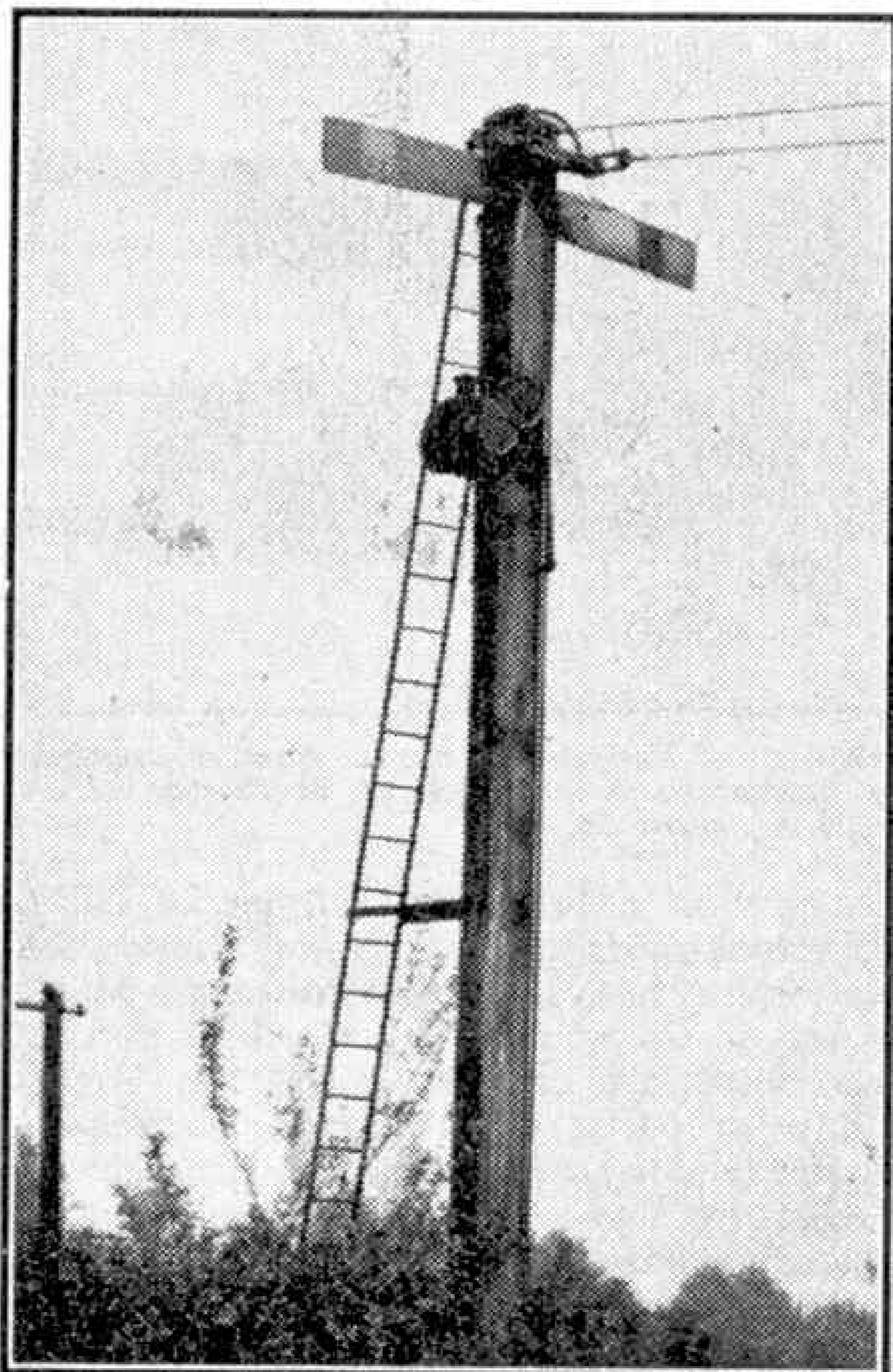
One lamp serves the spectacles for both semaphores on this old-type signal in which the arms move inside the slotted post.
