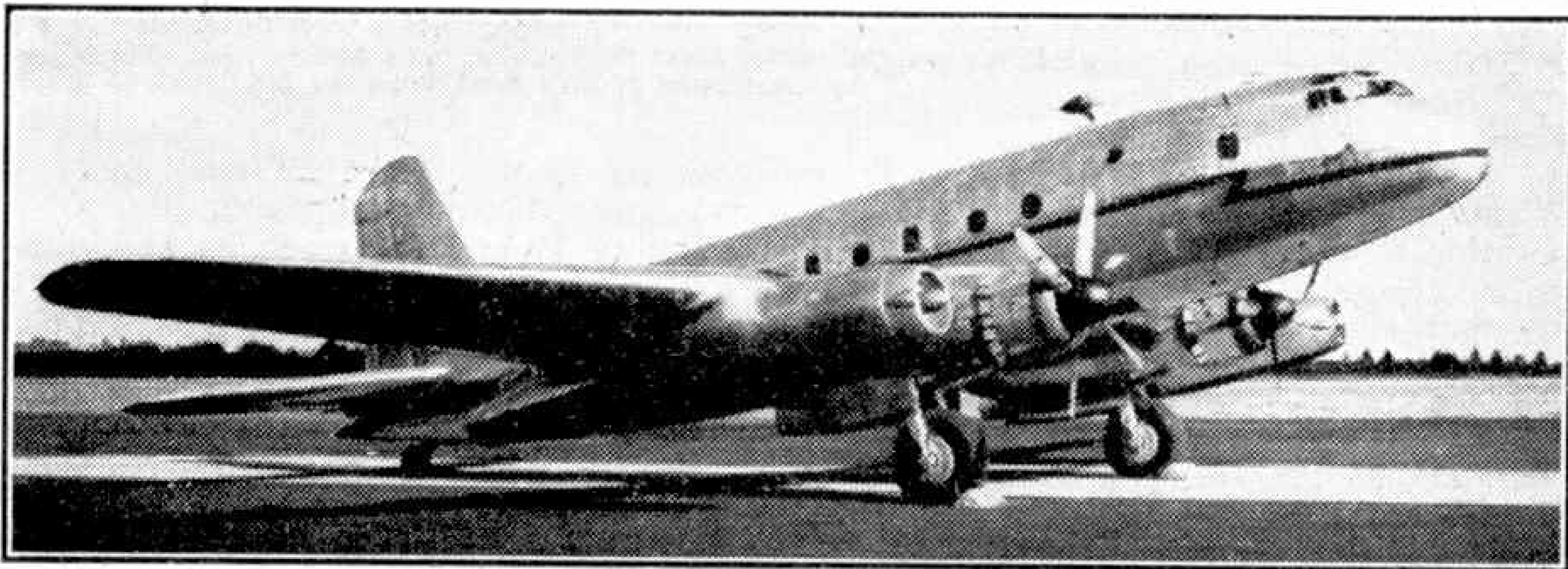
Handley Page "Hastings" fitted experimentally with two Armstrong-Siddeley "Sapphires," the world's most powerful turbo-jets, in place of its outboard pair of "Hercules." Photograph by courtesy of Handley Page Ltd.
