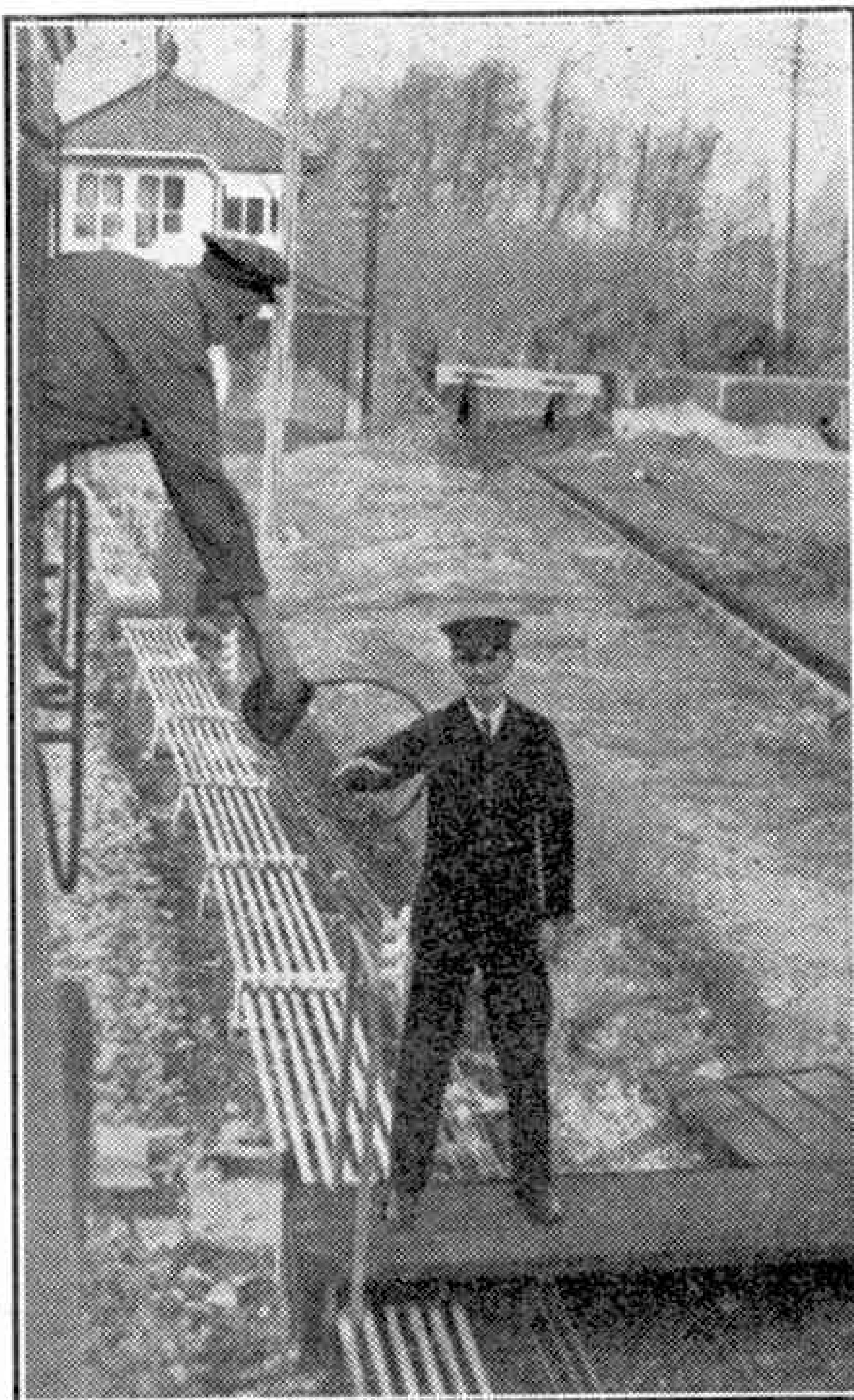
The driver of a push-and-pull unit leans out to hand over the tablet pouch to the waiting signalman.
