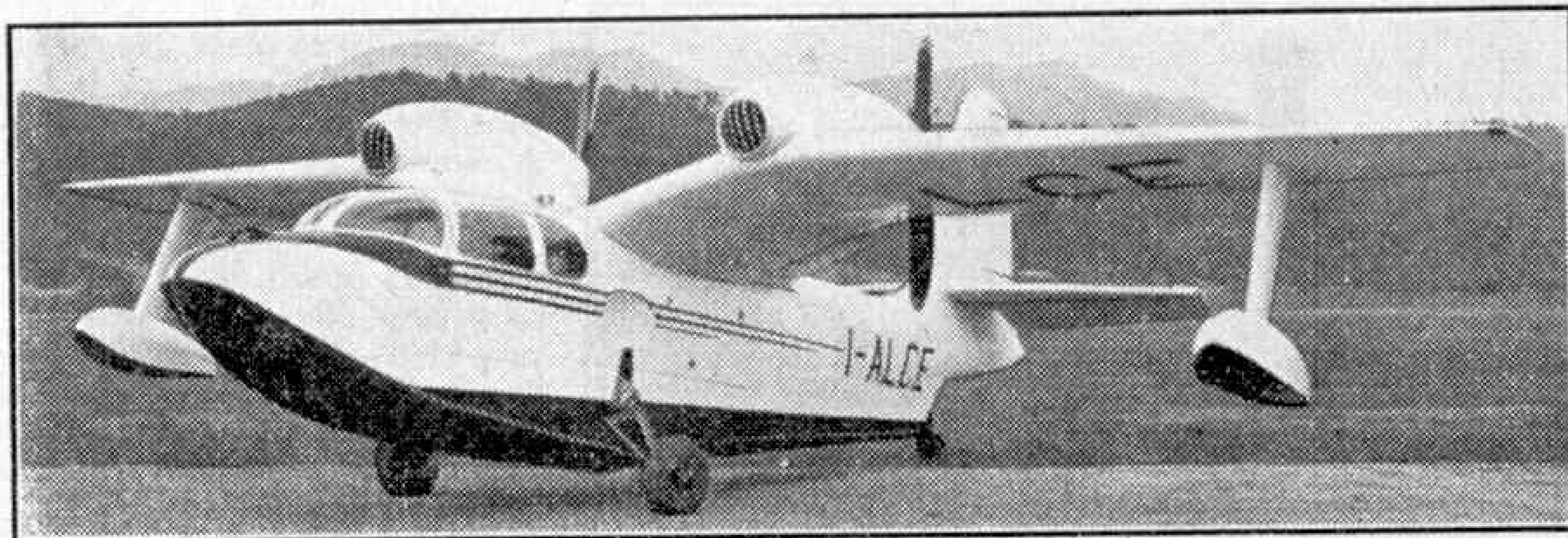
The Piaggio P.136 amphibian, showing the retractable undercarriage and the wing-tip floats. Photograph by courtesy of Piaggio and Company, Geneva.
