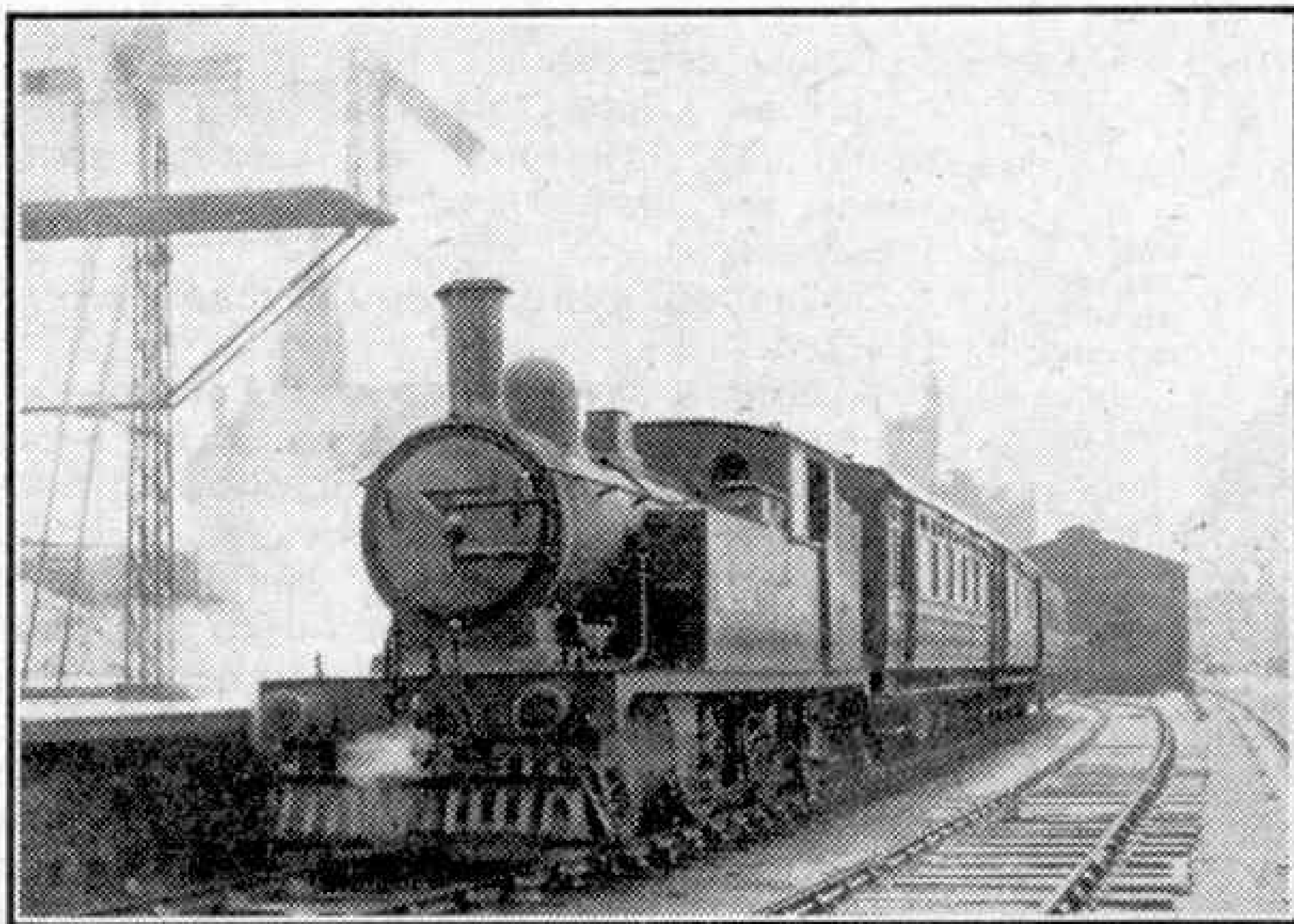
A "cowcatcher" on a B.R. locomotive? This photograph by J. N. Westwood, Mumbles, shows No. 67164, an ex-G.E. 2-4-2T, specially fitted for working the St. Combs Light Railway, in Aberdeenshire.
