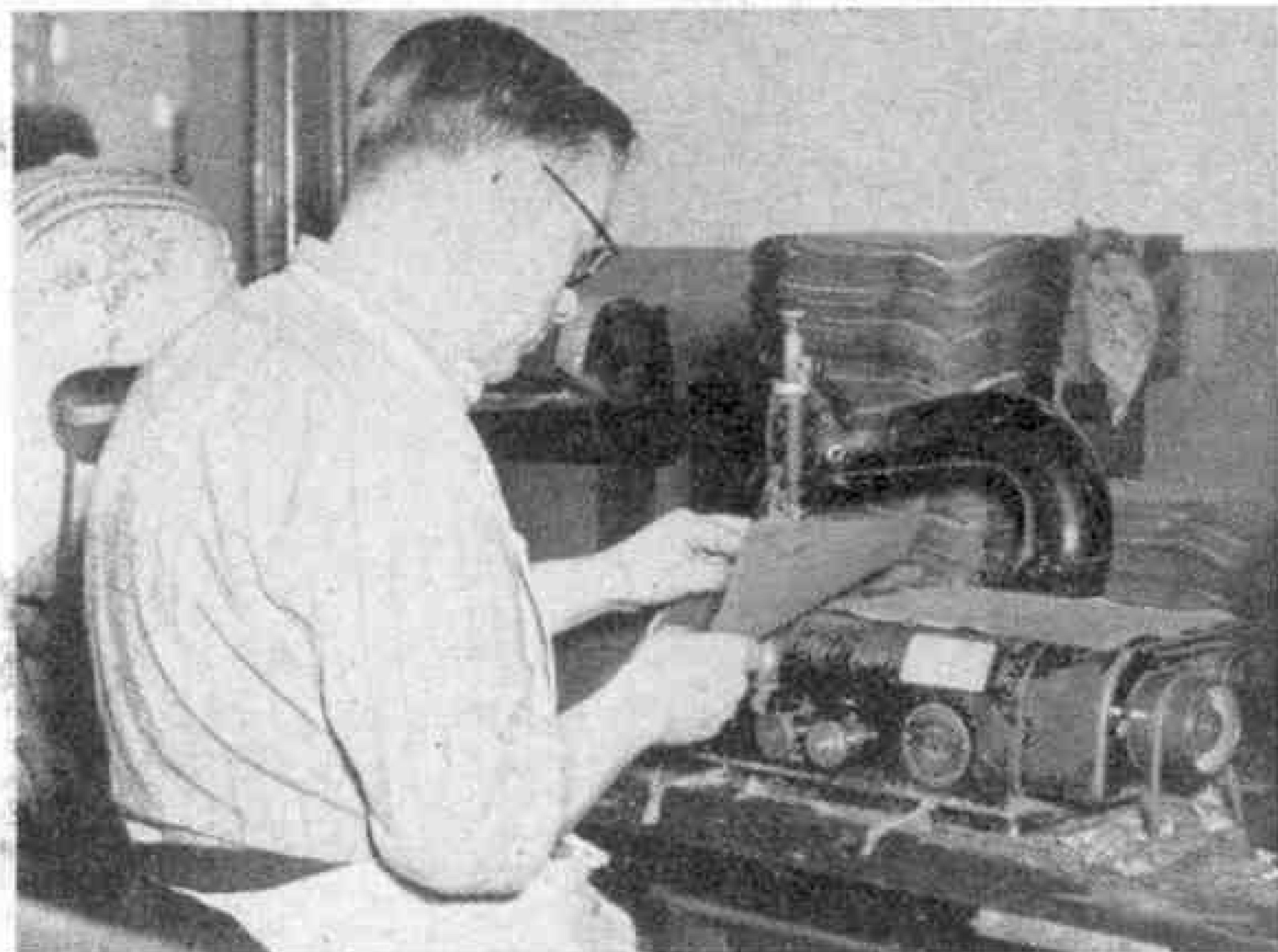
The craftsman at work here is skiving leather, that is paring it to half thickness at the edges to allow for turning these over when making up into binding cases for diaries.
