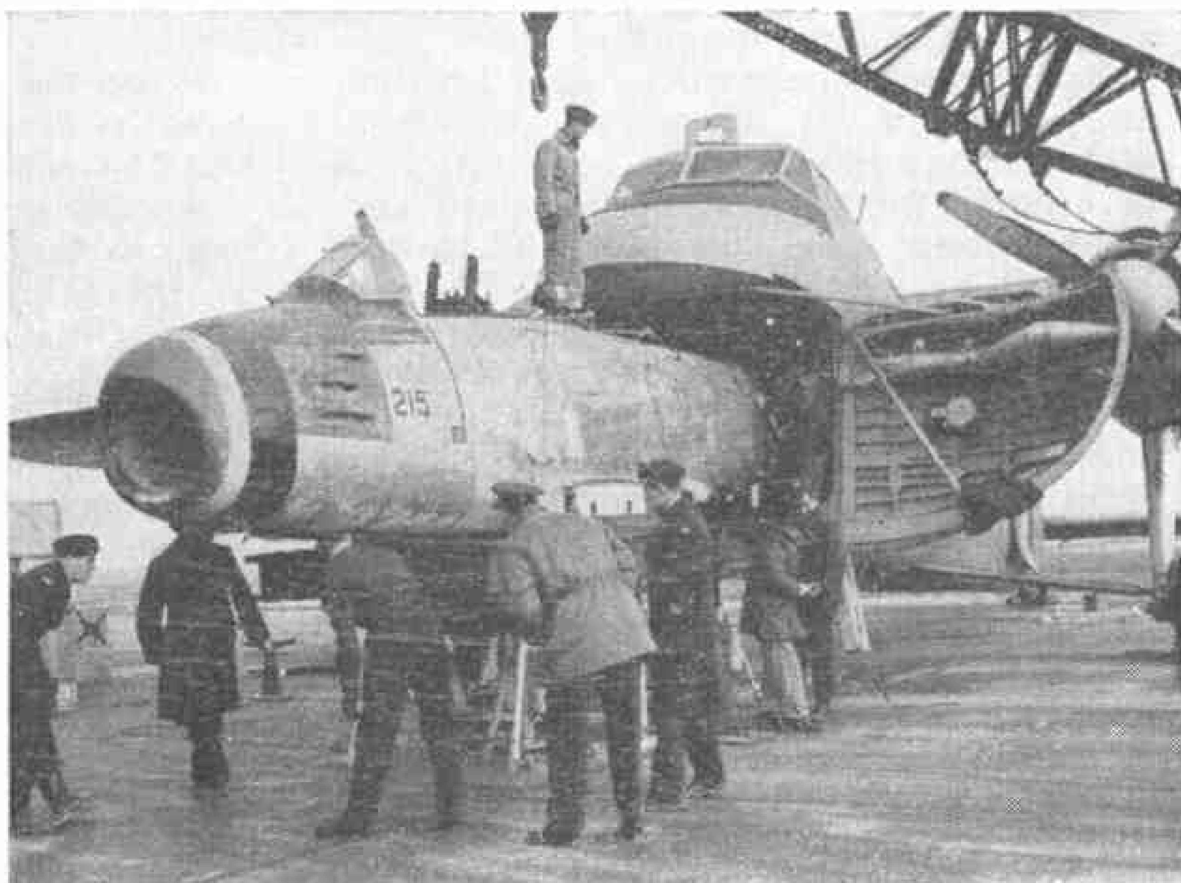
Loading a damaged Sabre jet fighter into a R.C.A.F. Bristol Freighter. Photograph by courtesy of Royal Canadian Air Force.
