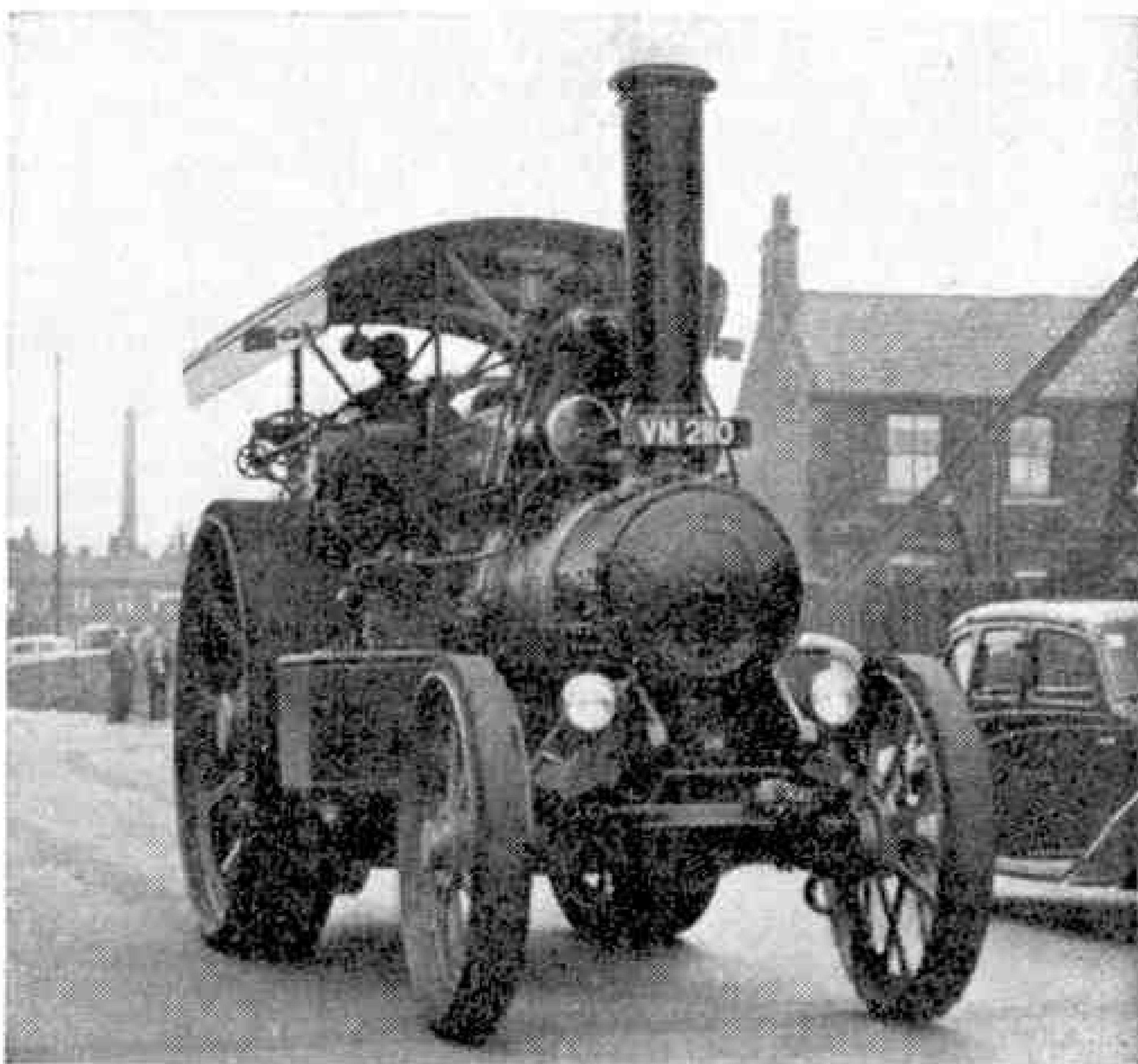
Atlas, a Fowler road engine completed in April 1928. It is equipped with a dismountable jib crane, the winding drum for which is seen on the off side, just forward of the top of the rear wheel. Photograph by courtesy of S. Mustill, Huyton, the present owner of Atlas.
