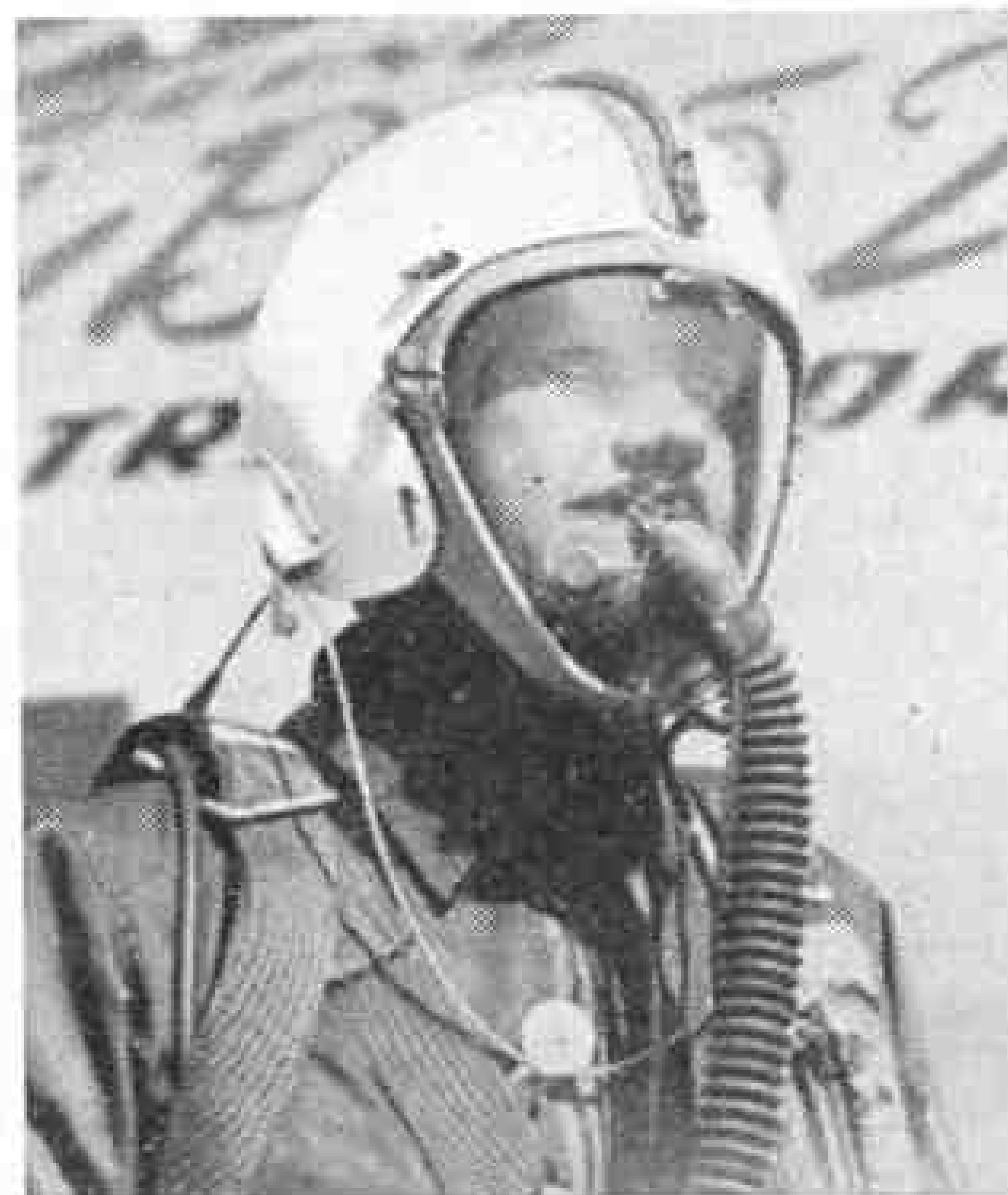
The helmet of the new U.S.A.F. high-altitude emergency pressure suit.
