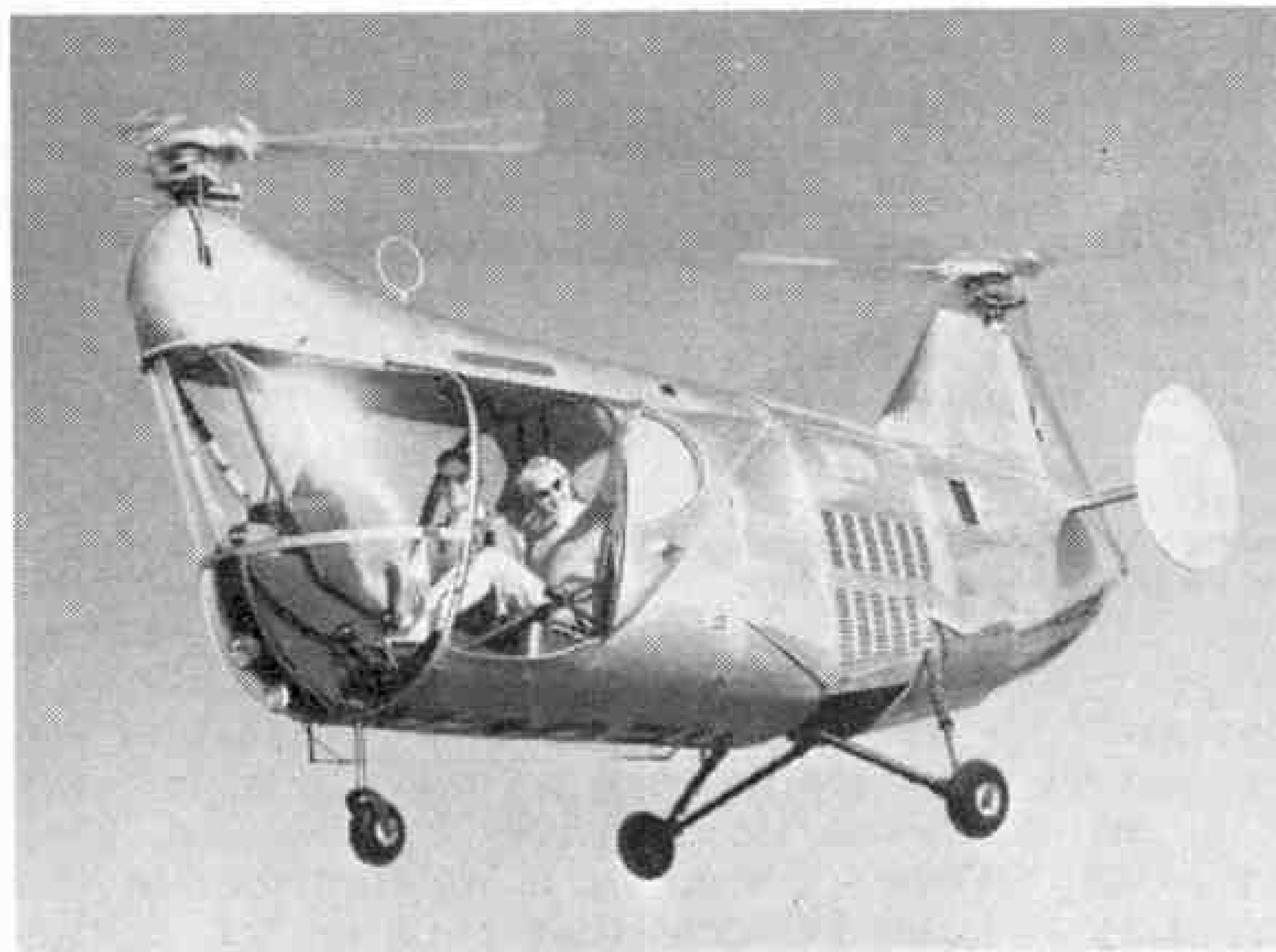
The McCulloch MC-4, the first tandem-rotor helicopter to be licensed in the United States for commercial use, carries its first civilian passenger. Photograph by courtesy of McCulloch Motors Aircraft Division, U.S.A.
