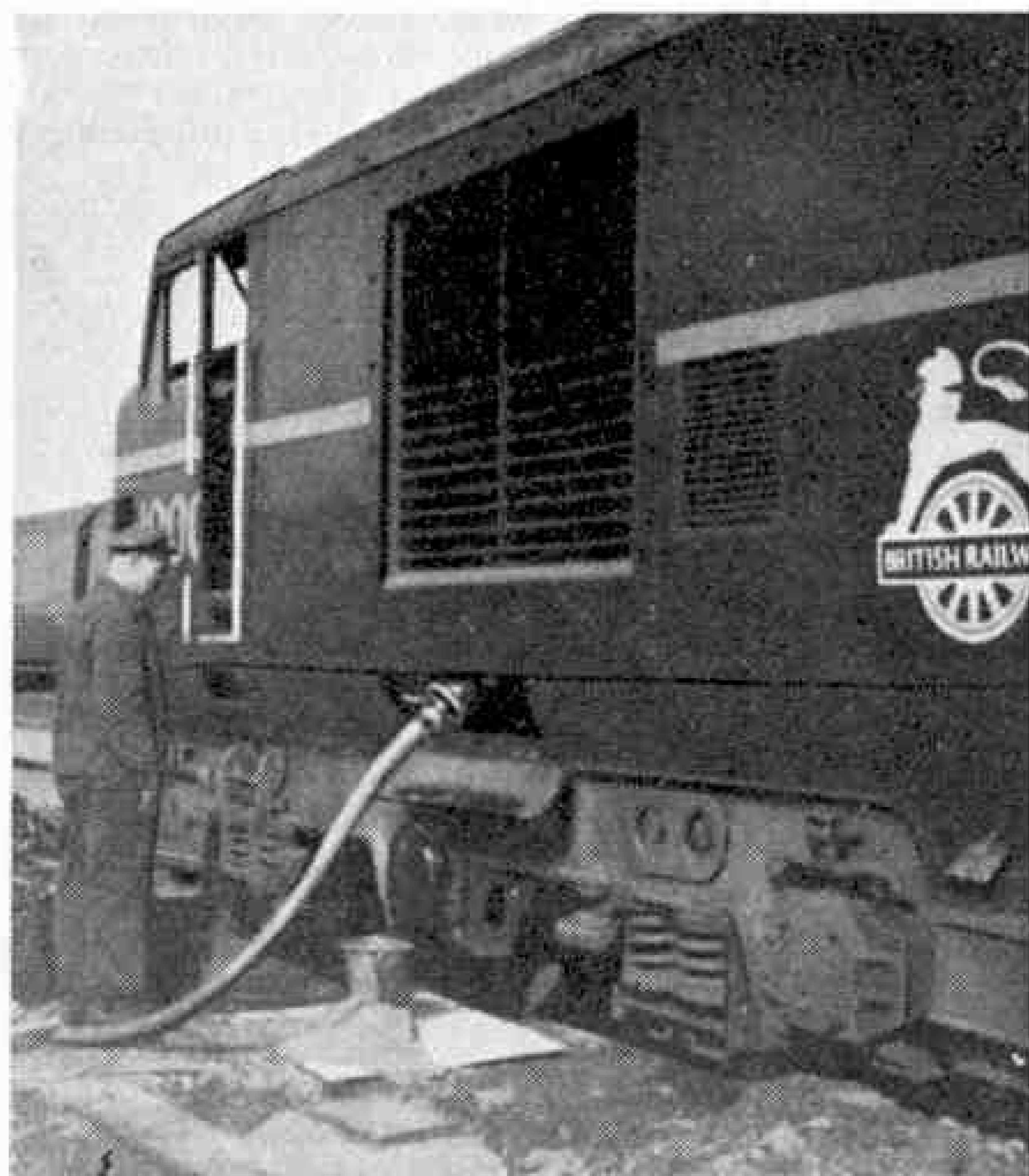
Filling the fuel tanks of No. 10000 at Windsor Sidings, Waterloo. Photographs by the author.
