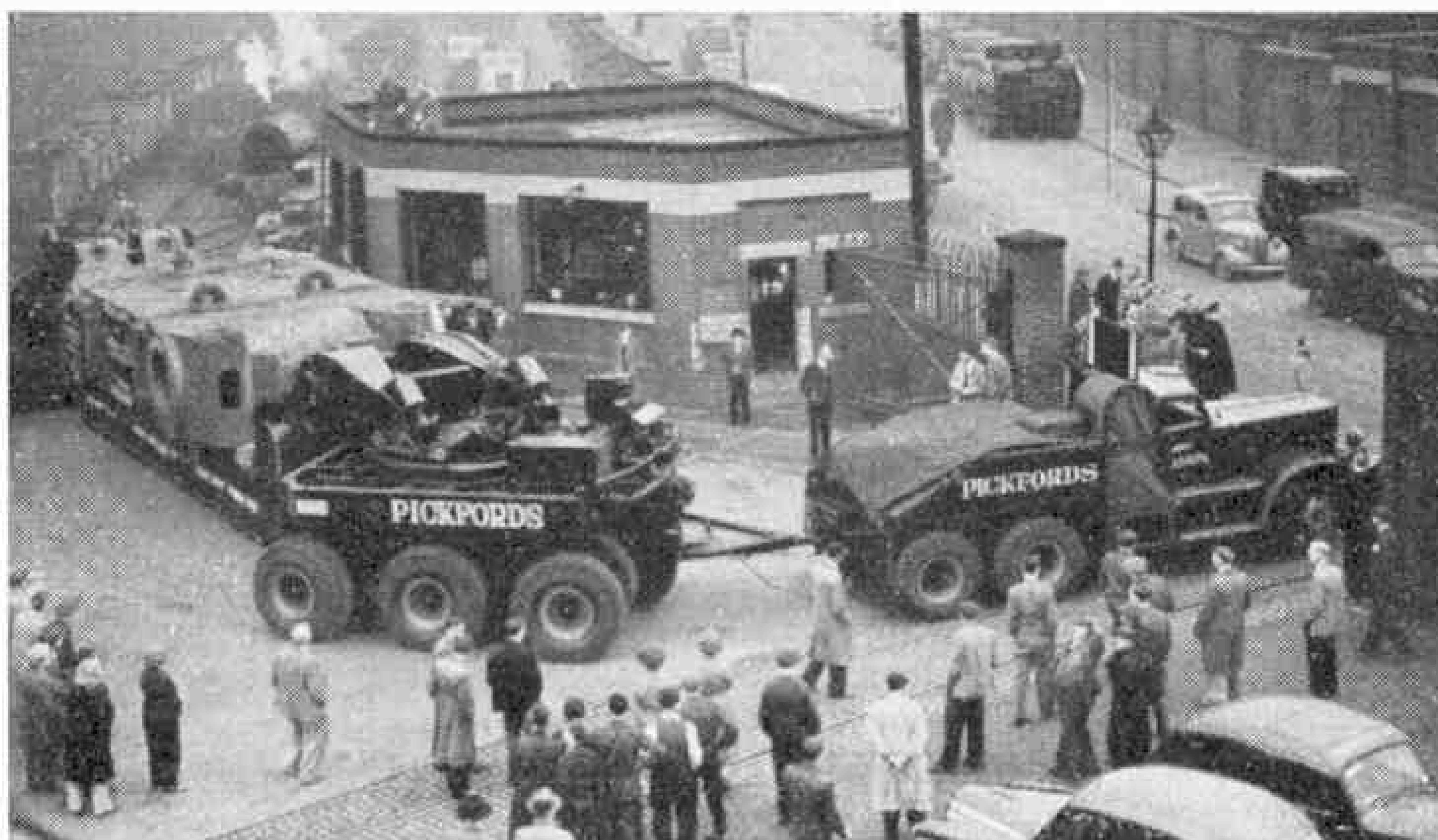
Hauling a casting weighing 164 tons on the Crane 200-ton trailer. This photograph, reproduced by courtesy of Kemsley Newspapers Ltd., shows how the swan necks rest on the turntables of the bogies.
