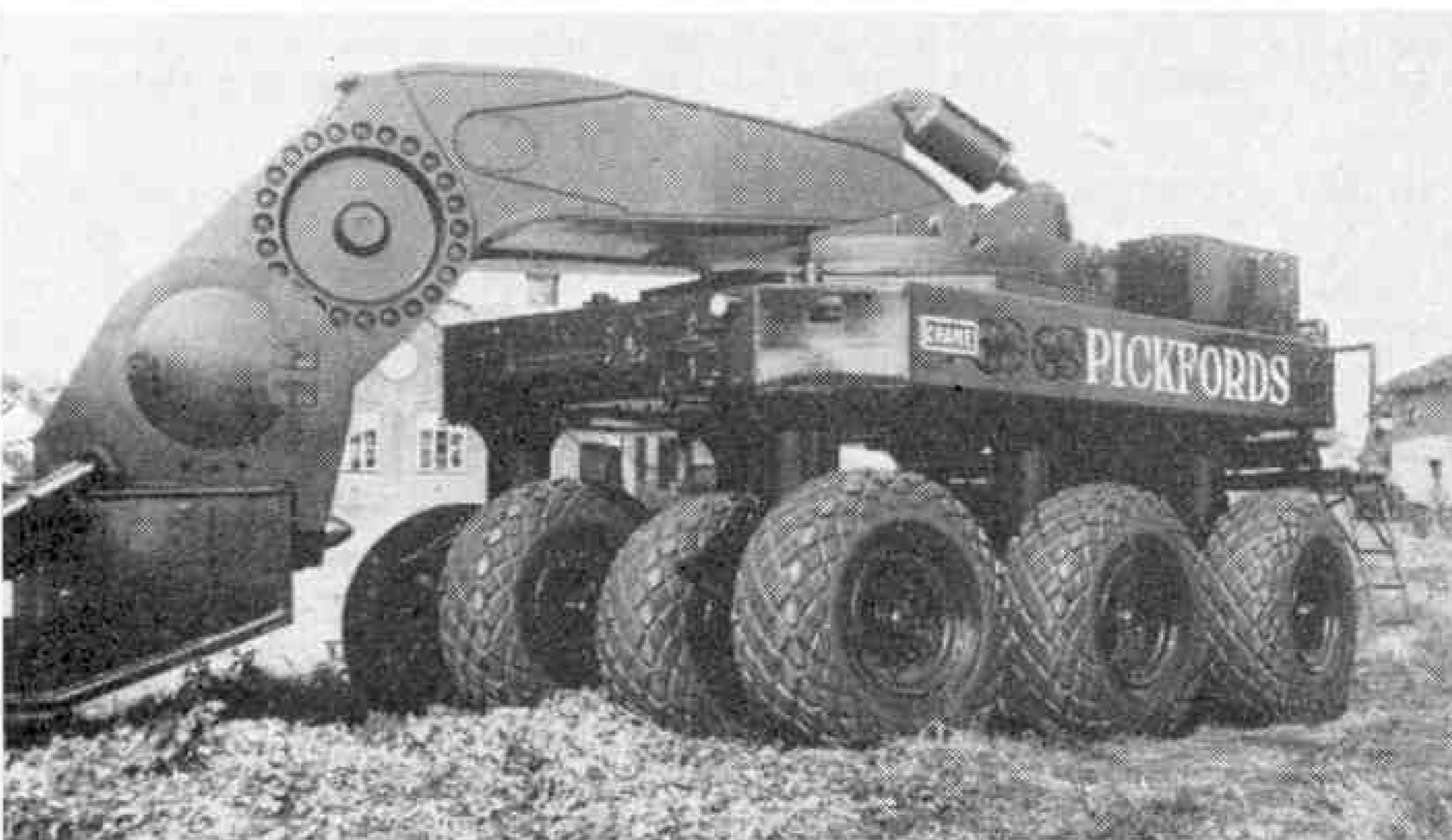
A bogie and swan neck of a giant among trailers, the Crane 200-ton transporter, the largest of its kind in the world.
