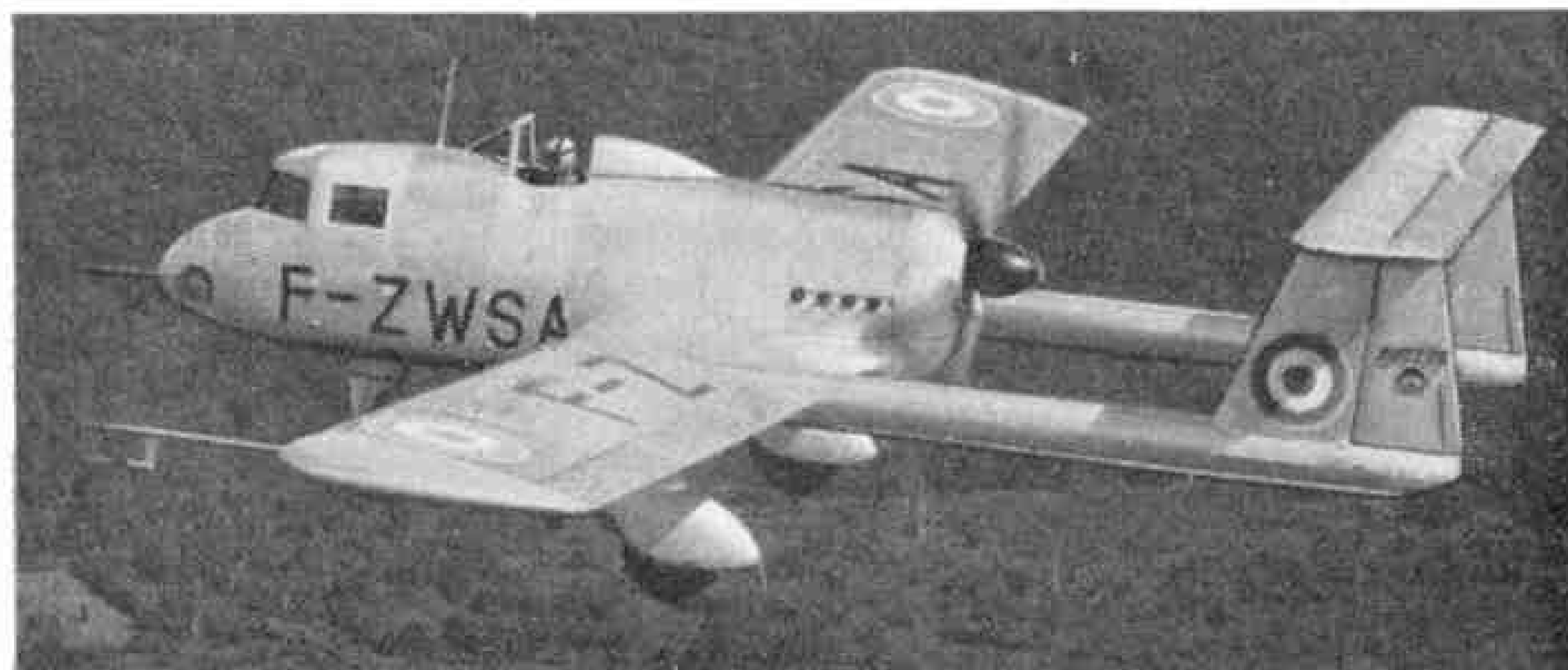
Potez 75. This interesting "battling bantam" type has a 450 h.p. "pusher" engine and a fixed undercarriage.
