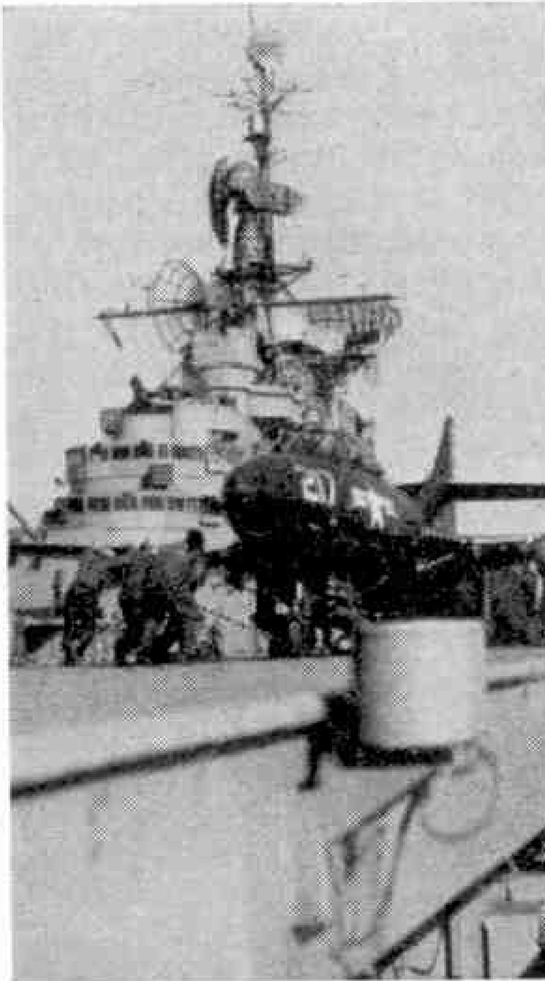
Panther jet fighter being prepared for catapulting as a Douglas Skyraider takes off from the angled flight deck.
