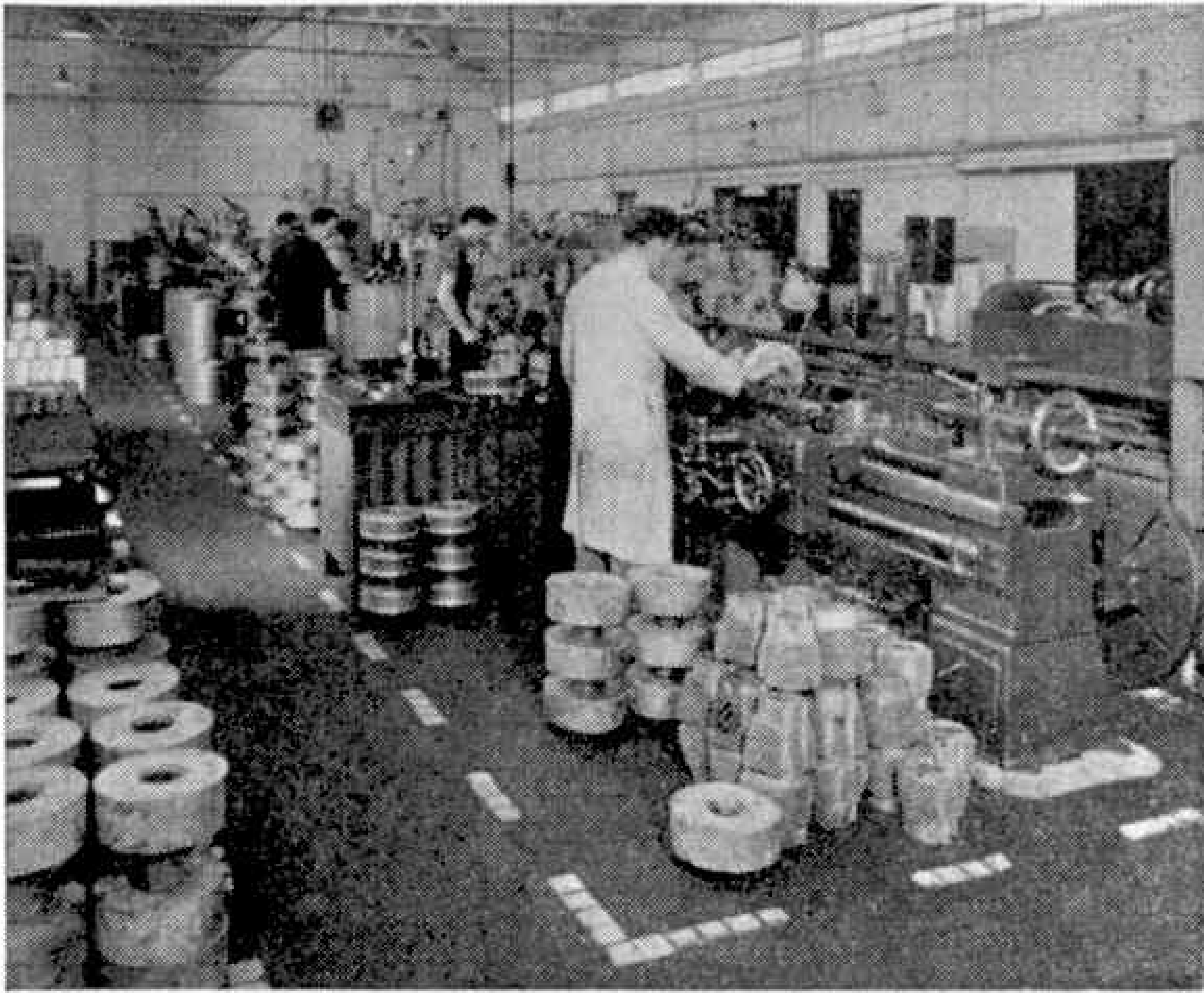
Wellworthy Al-fin cylinder barrels being machined.
