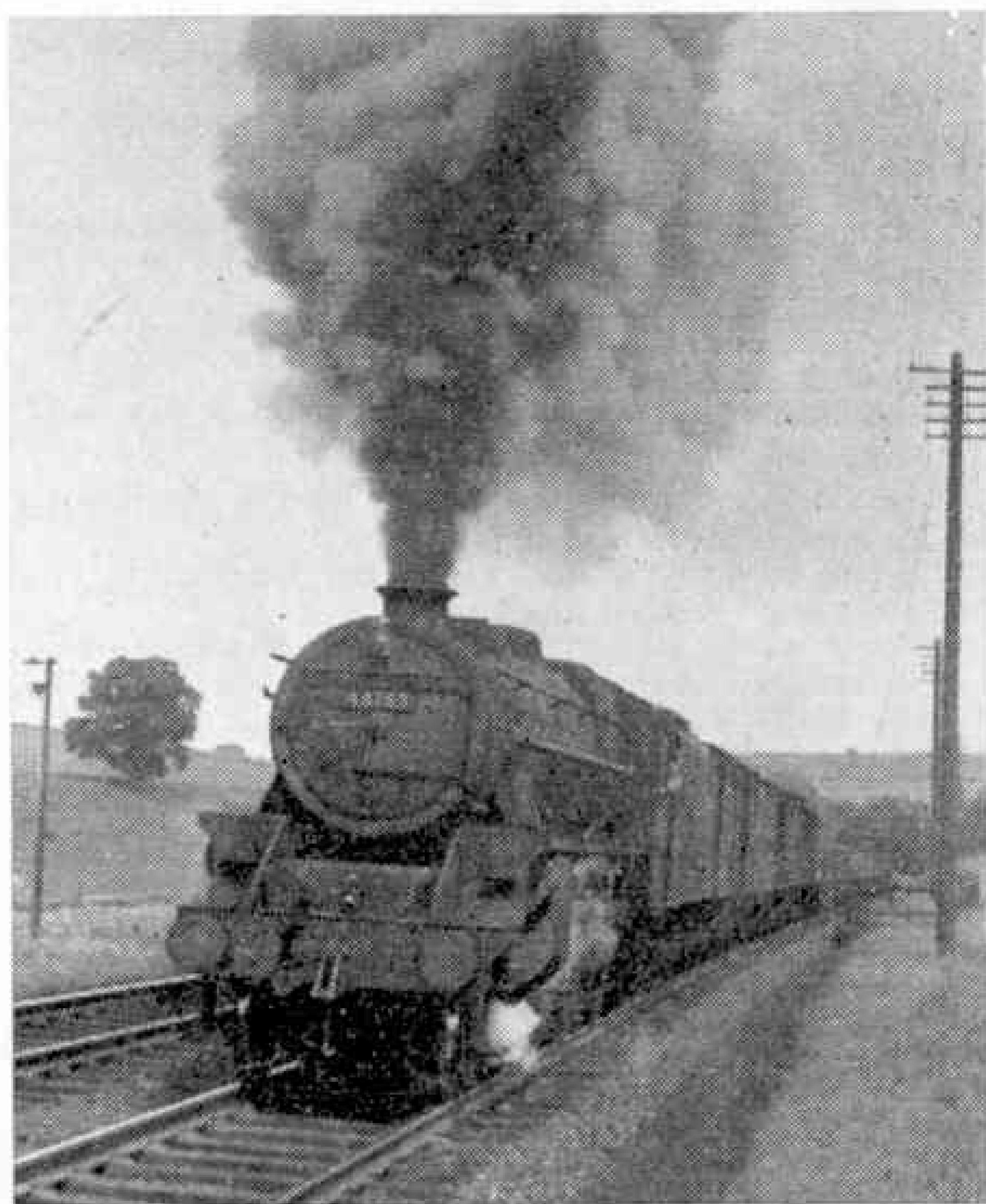
A London Midland fast freight train near Thrimby on the Northern ascent to Shap summit. The engine is one of the familiar Stanier class 5 mixed traffic 4-6-0s No. 44763. Photograph by Archdeacon E. Treacy.
