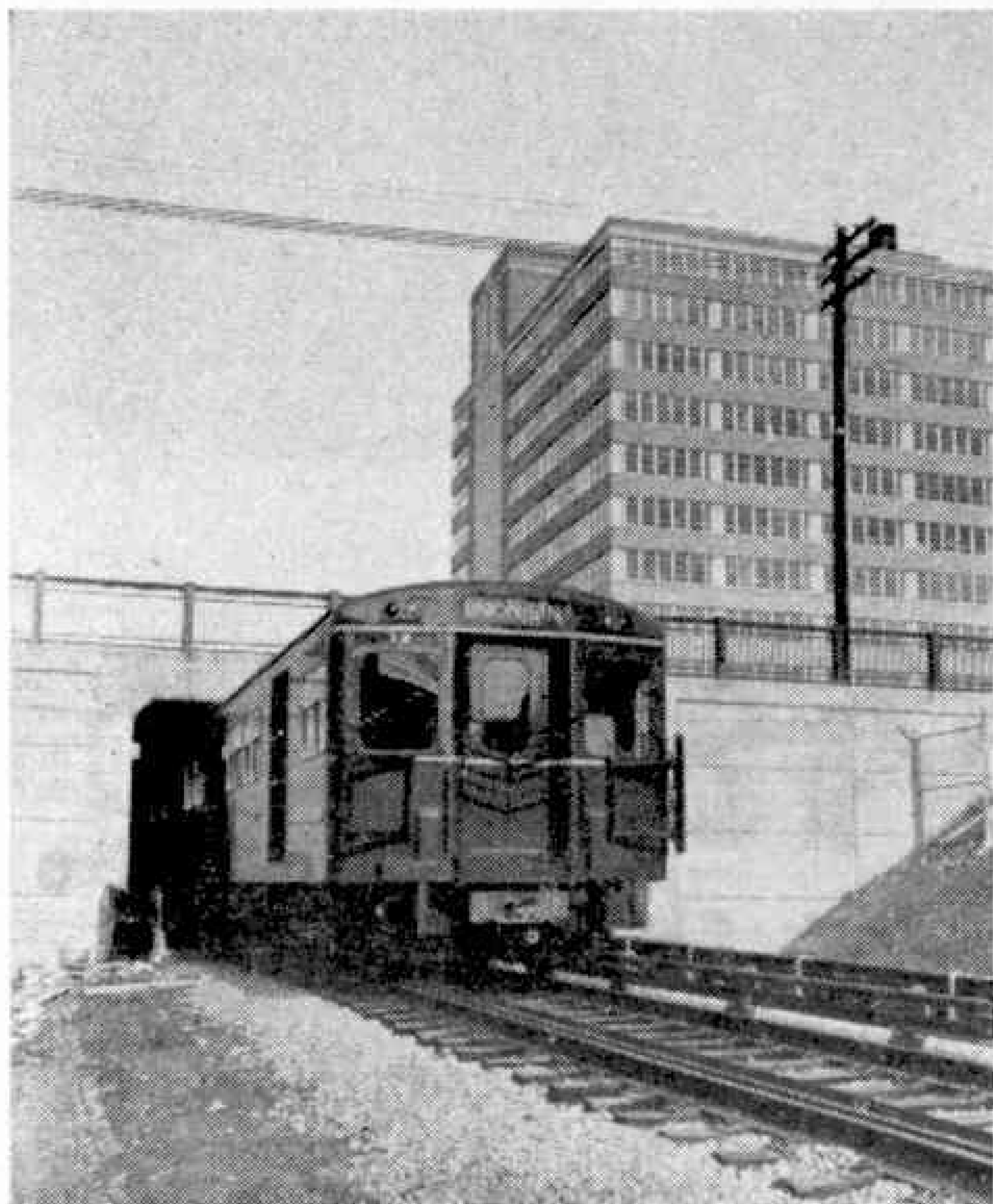
One of the British-built subway trains coming from an underground section into an open cut section near the maintenance yards.
