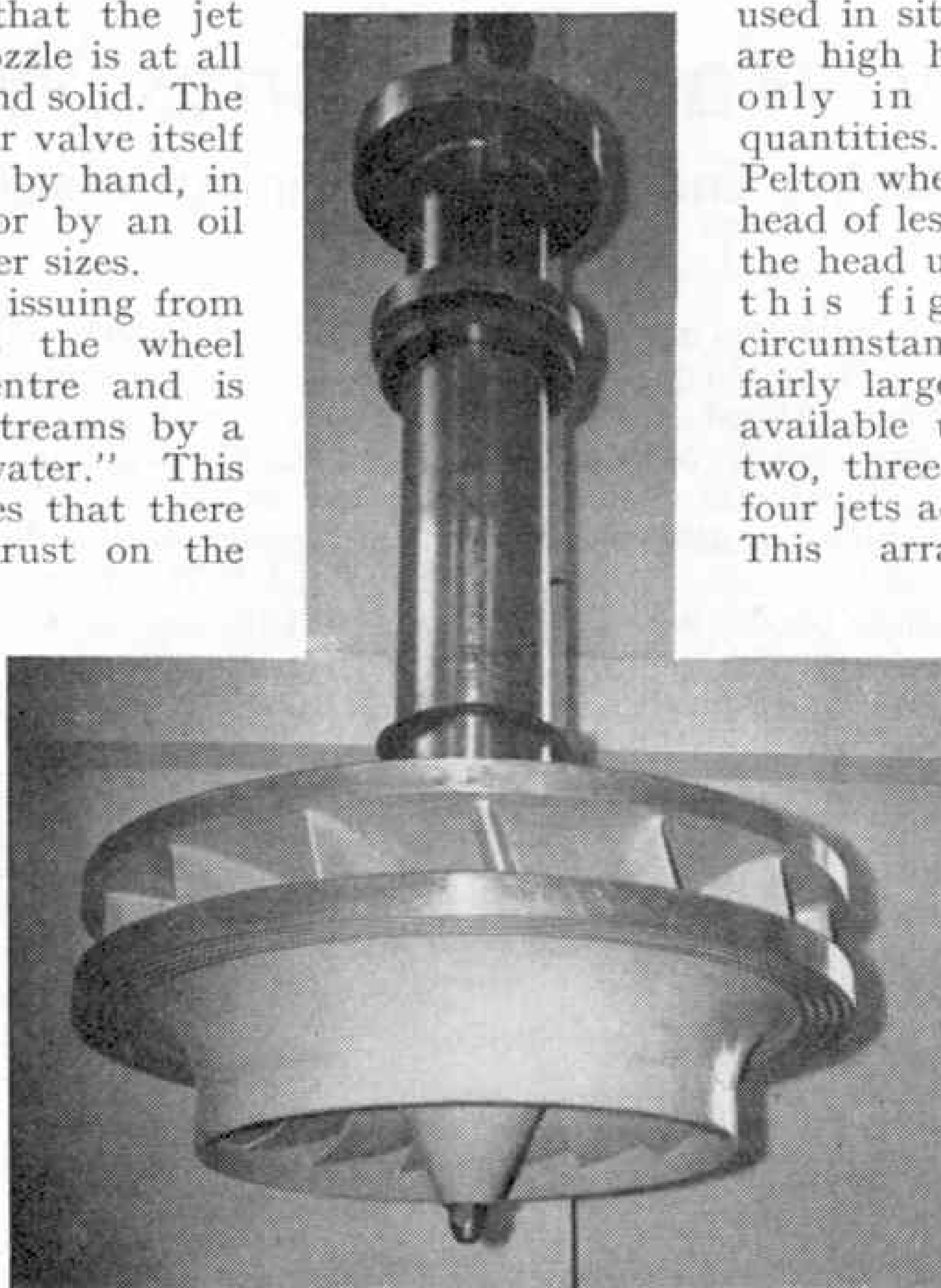
The runner of a Francis turbine. This is a reaction turbine, the water "pushing" the runner round.
