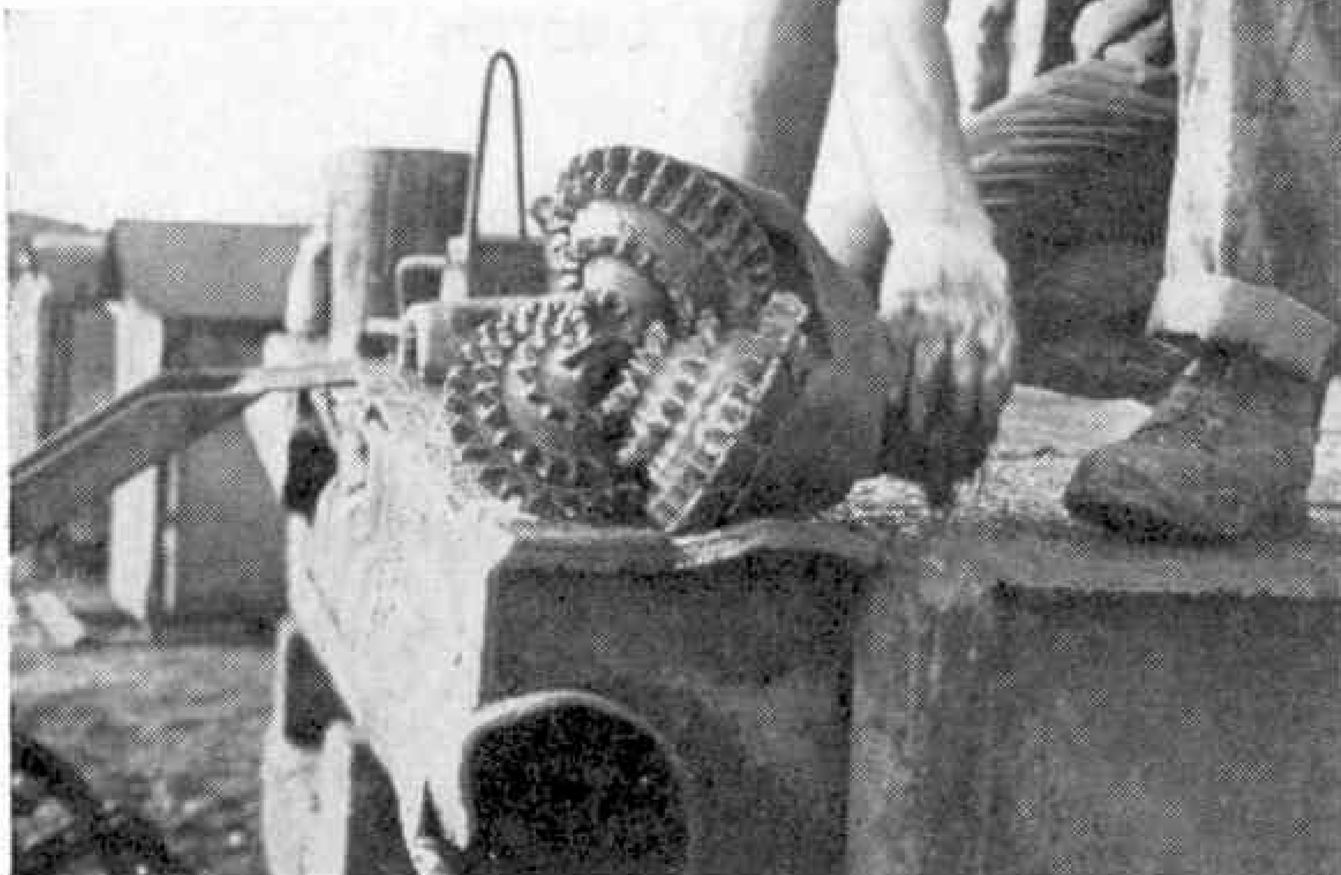
The tri-cone drilling rock bit used in drilling through hard formations.
