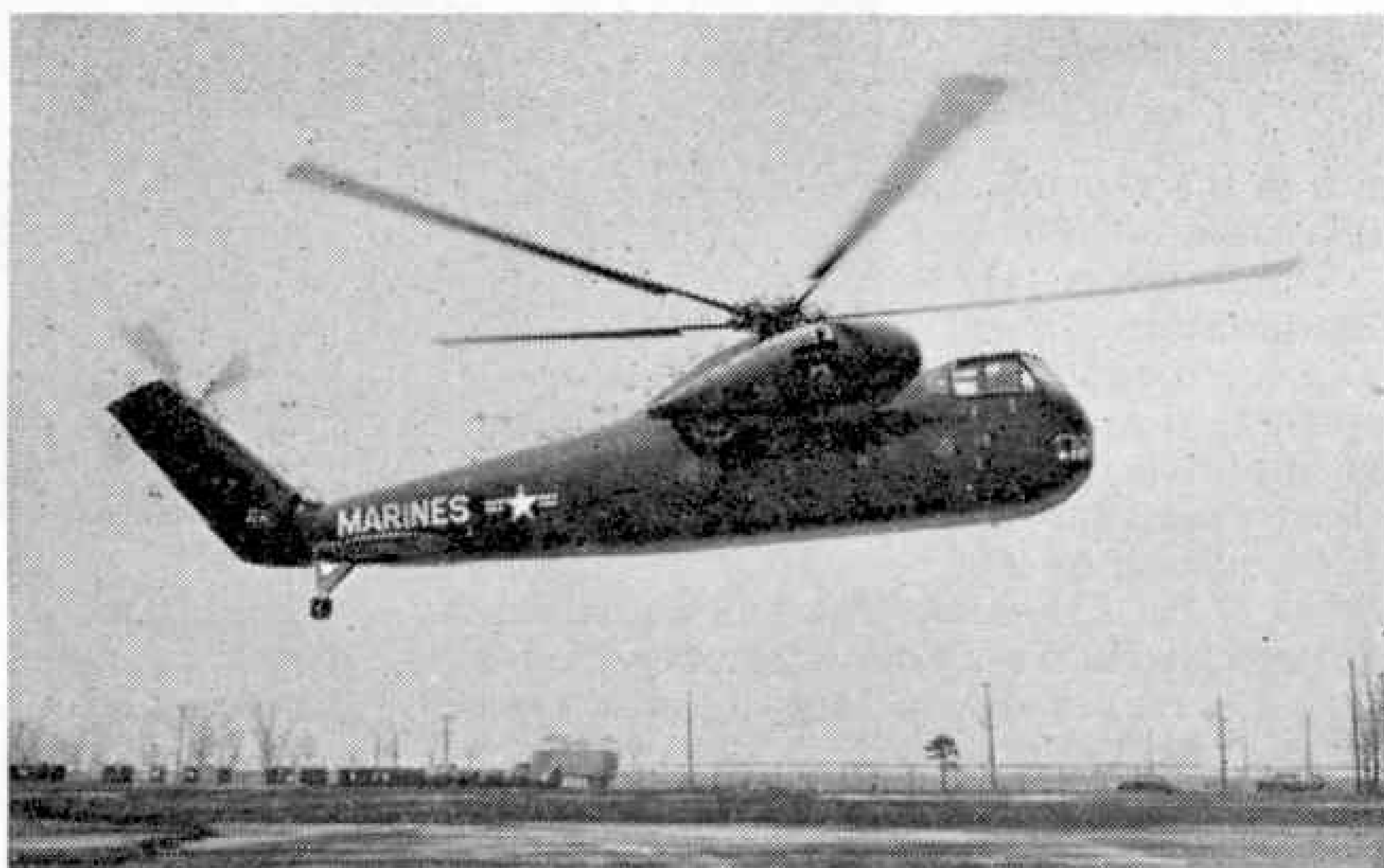
The new Sikorsky S-56 twin-engine helicopter, designed for the U.S. Marine Corps.
