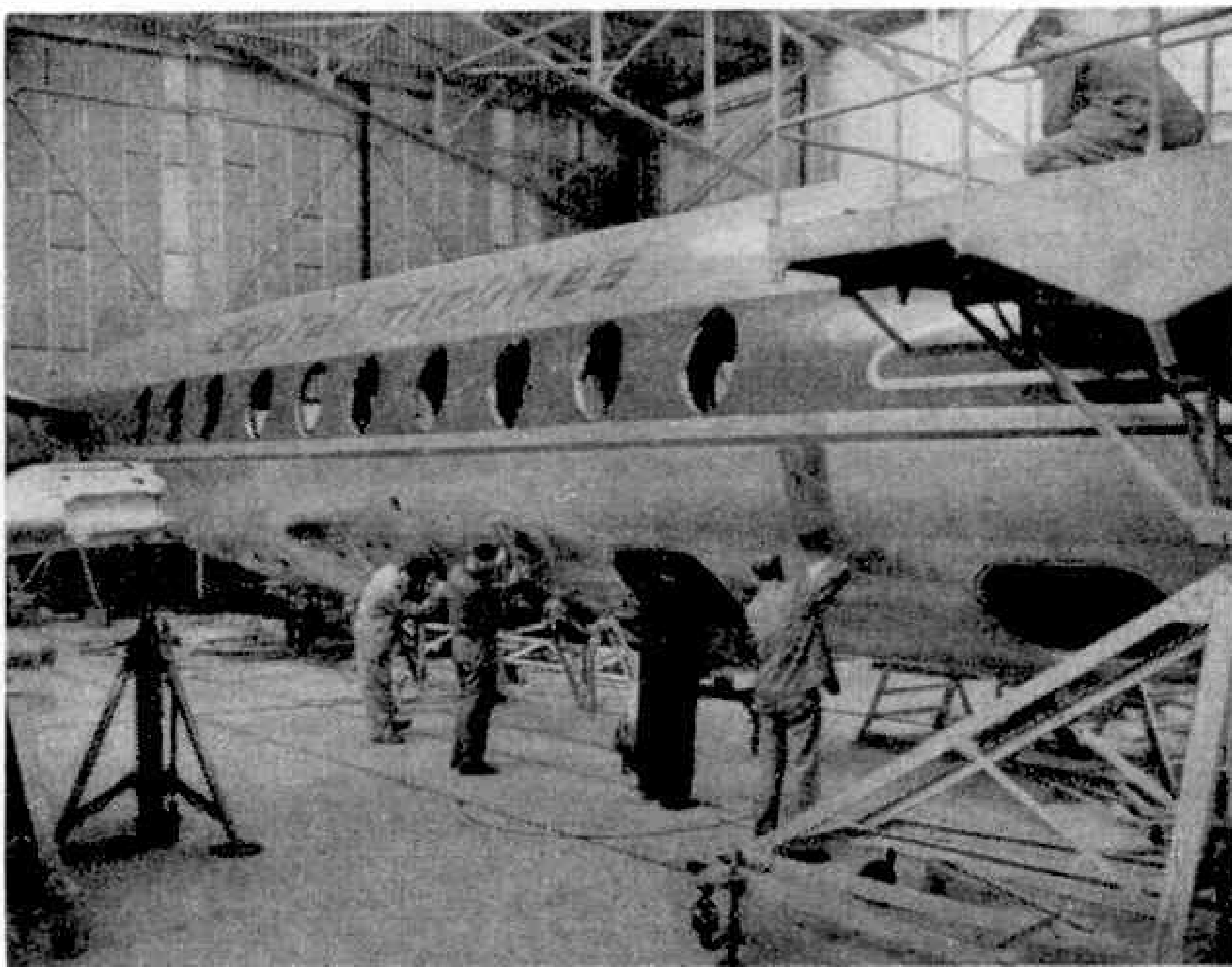
At work on the fuselage of one of the Viscount air liners for Capital Airlines, U.S.A. Photograph by courtesy of Vickers-Armstrongs Ltd.
