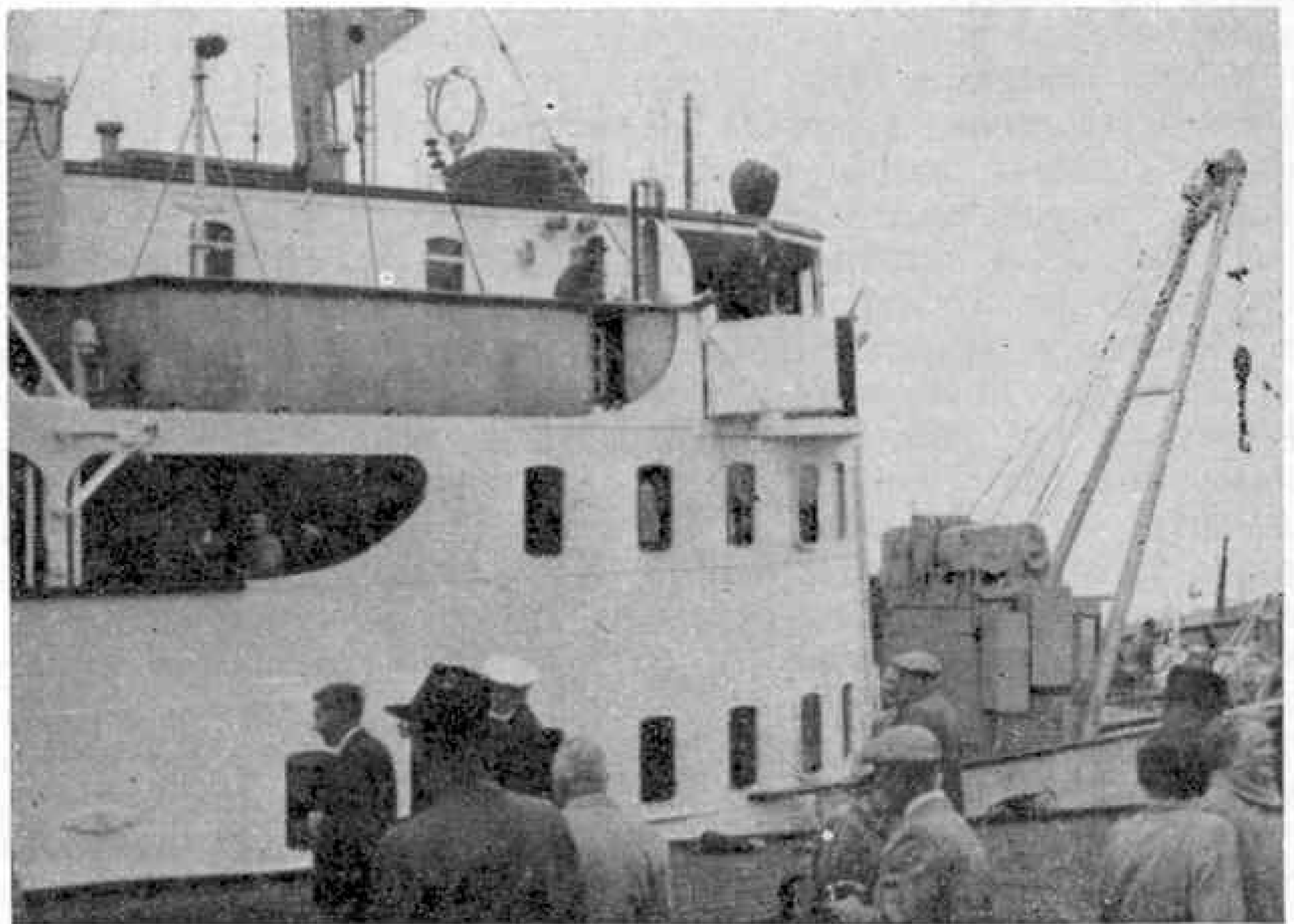
The "St. Ninian" at Leith. A powerful electric crane is mounted forward of the bridge.
