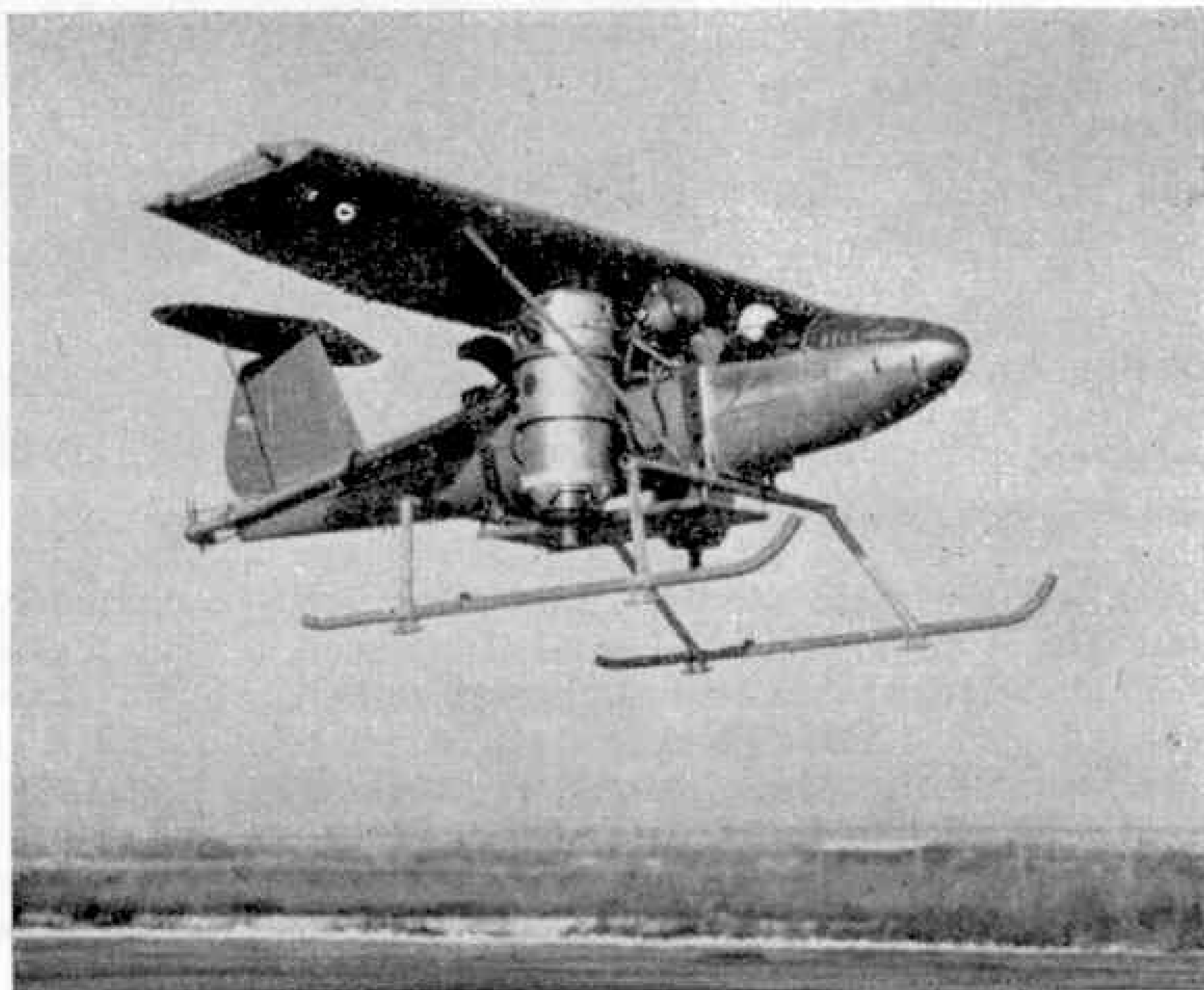
Another revolutionary Bell type, the VTOL (vertical take-off and landing) aircraft. It was built to prove the practicability of direct jet-lift.
