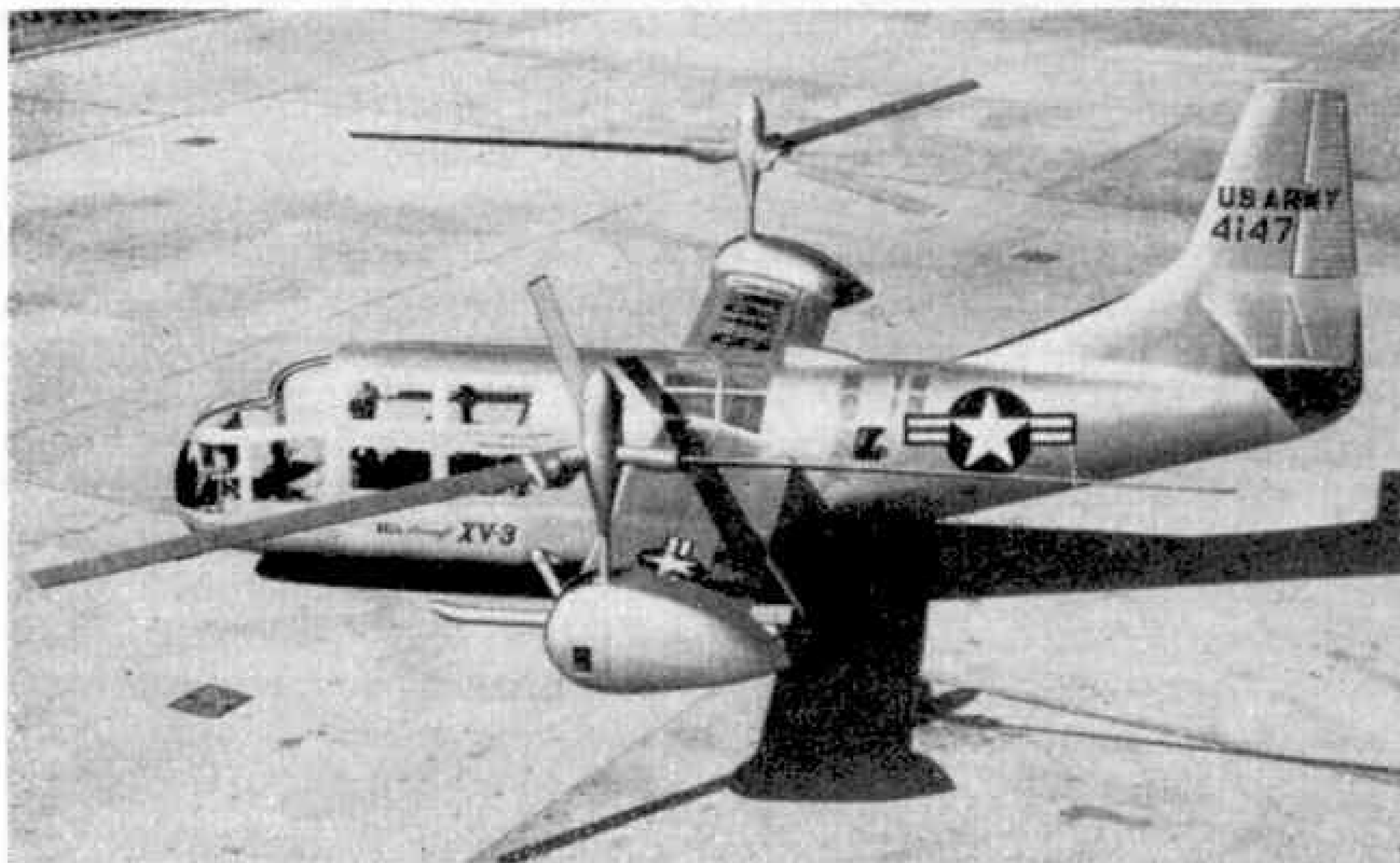
The Bell XV-3 Convertiplane, the two rotors of which are mounted at the wing-tips.
