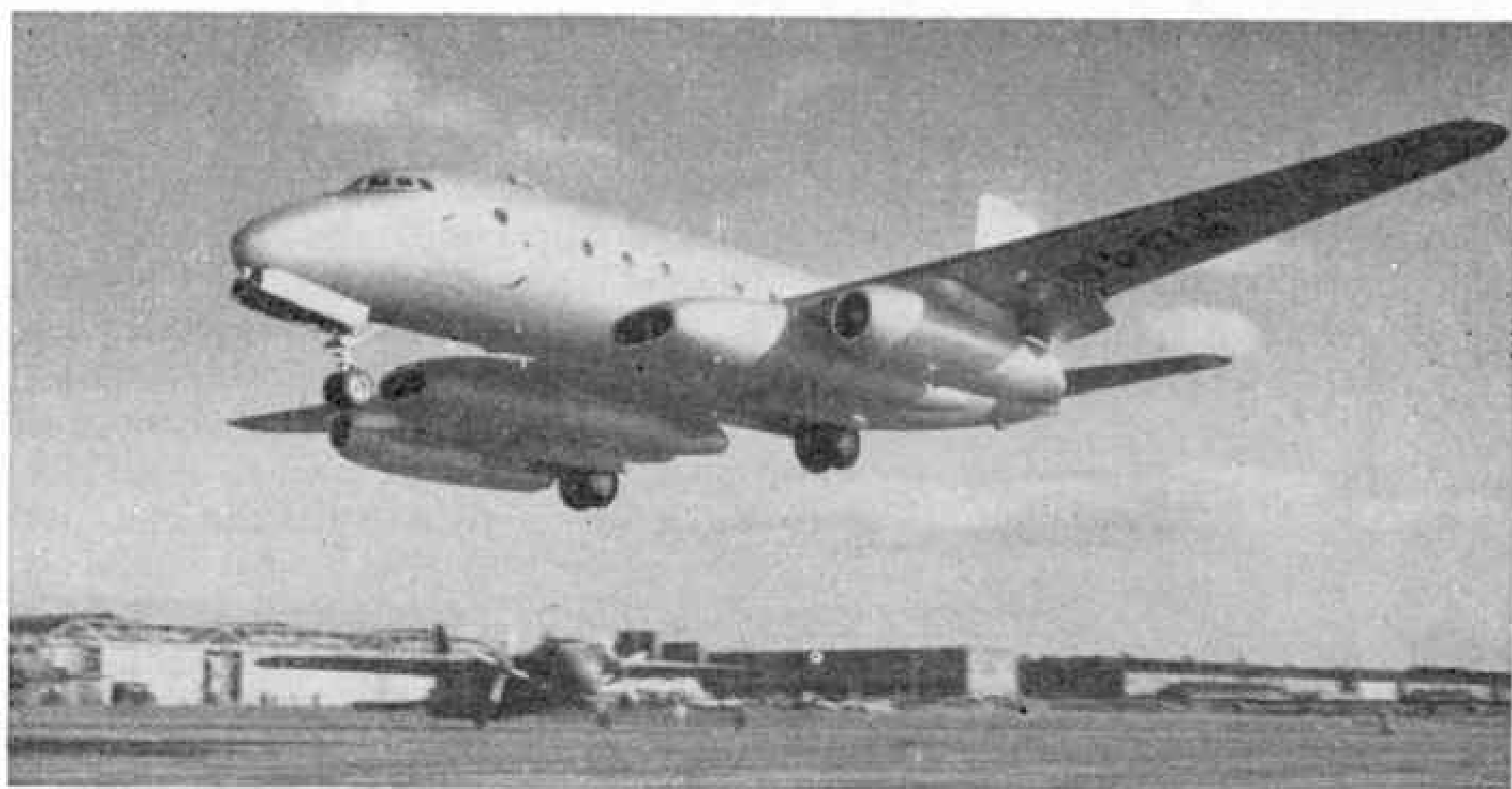
Avro Ashton, with its four Rolls-Royce Nene engines supplemented by two Bristol Olympus turbojets in pods under its wings.
