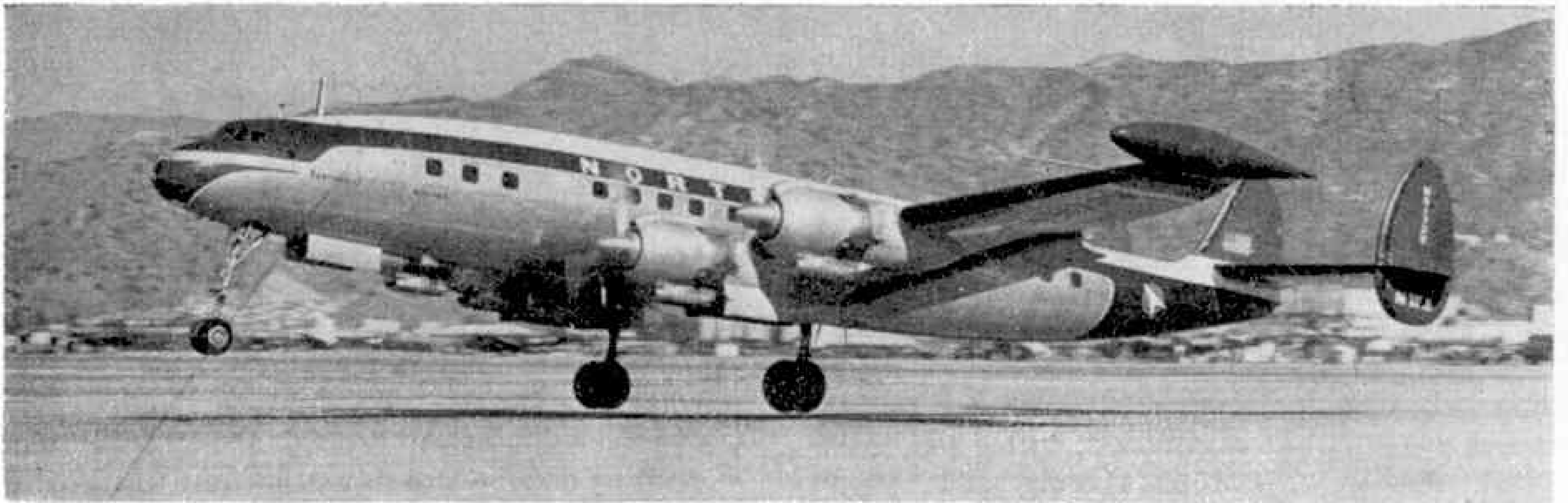
This Super Constellation of Northwest Orient Airlines, U.S.A., is the first civil air liner to be fitted with wing-tip fuel tanks to increase its range on scheduled services. It is shown taking off on a test flight.
