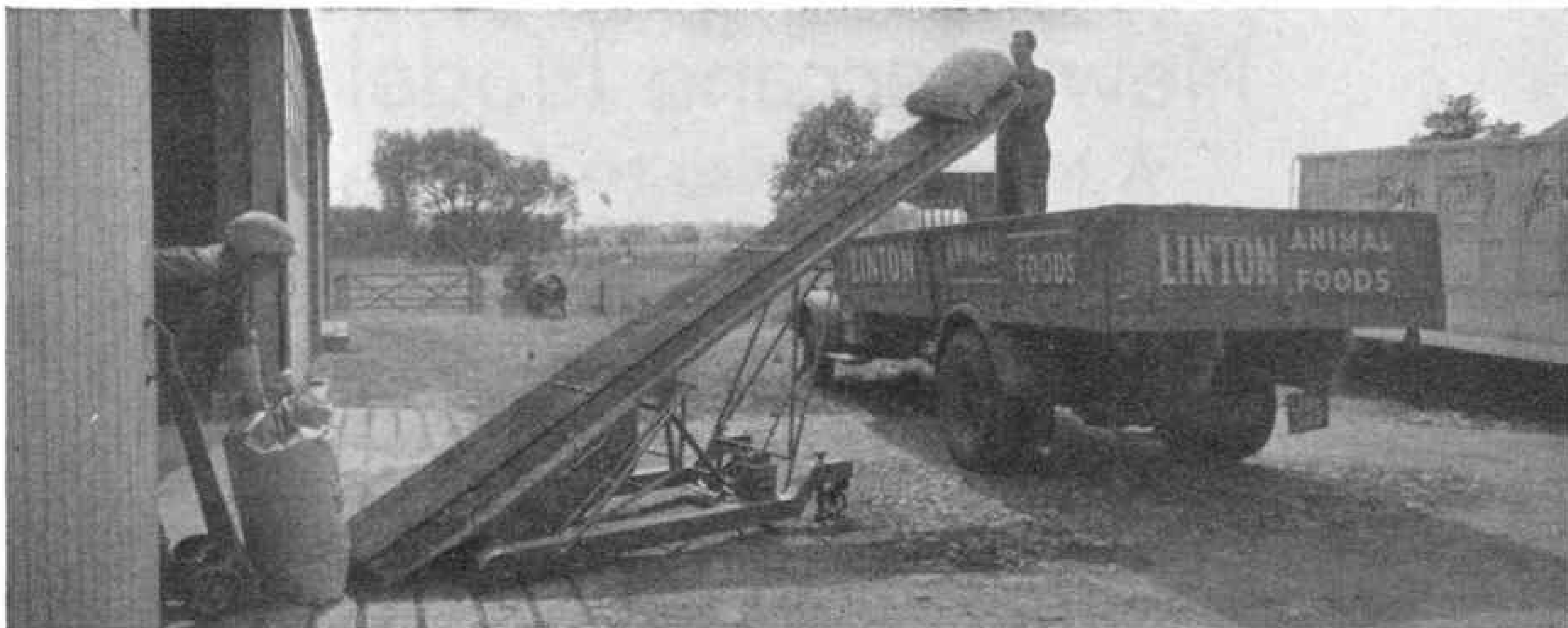
Fig. 2. The LoadaVeyor in action loading filled sacks from a warehouse into a motor lorry. Notice the upstands fixed across the belt to prevent the sacks slipping.
