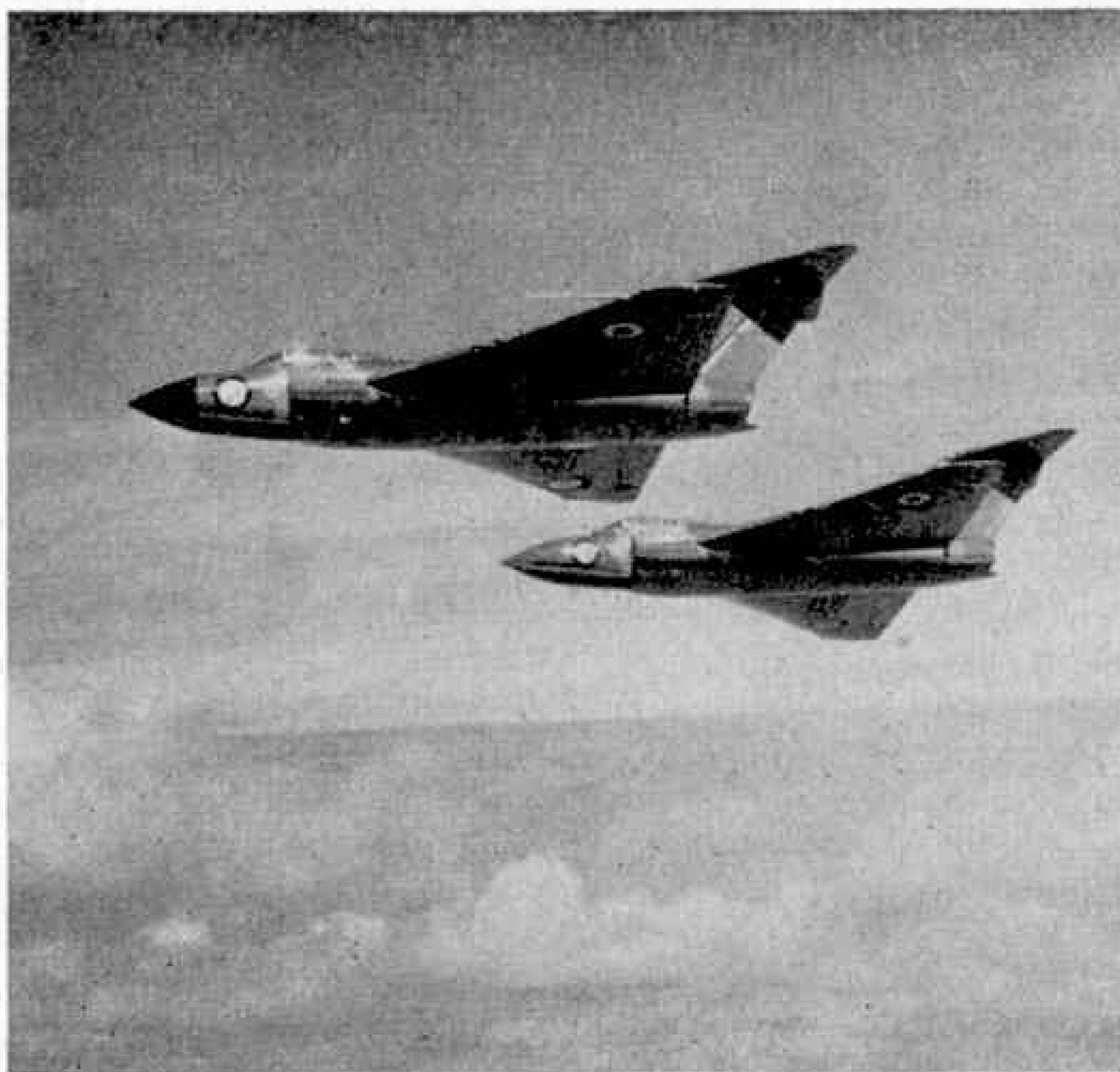
These Gloster Javelins for R.A.F. Fighter Command have a sharply-pointed cone over the radar scanner in the nose.
