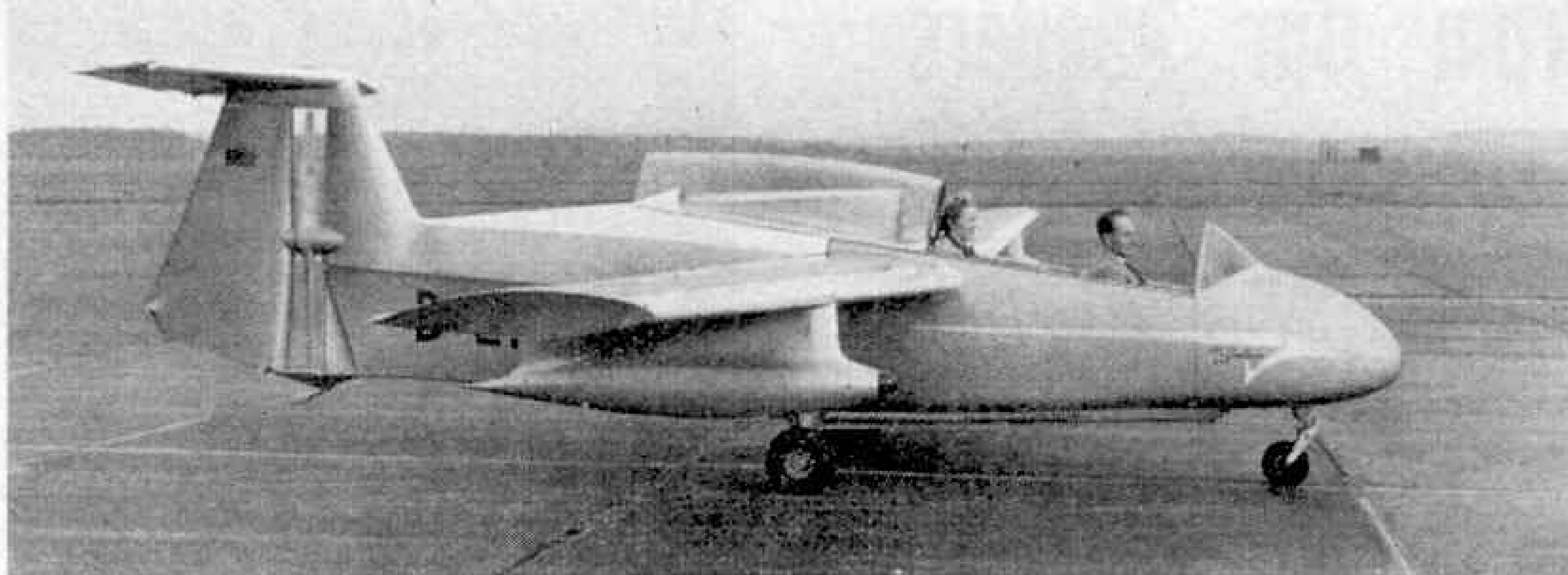
This unusual aircraft is the German-built RW3 Multoplane. The propeller is mounted in a slot between the fin and the rudder.
