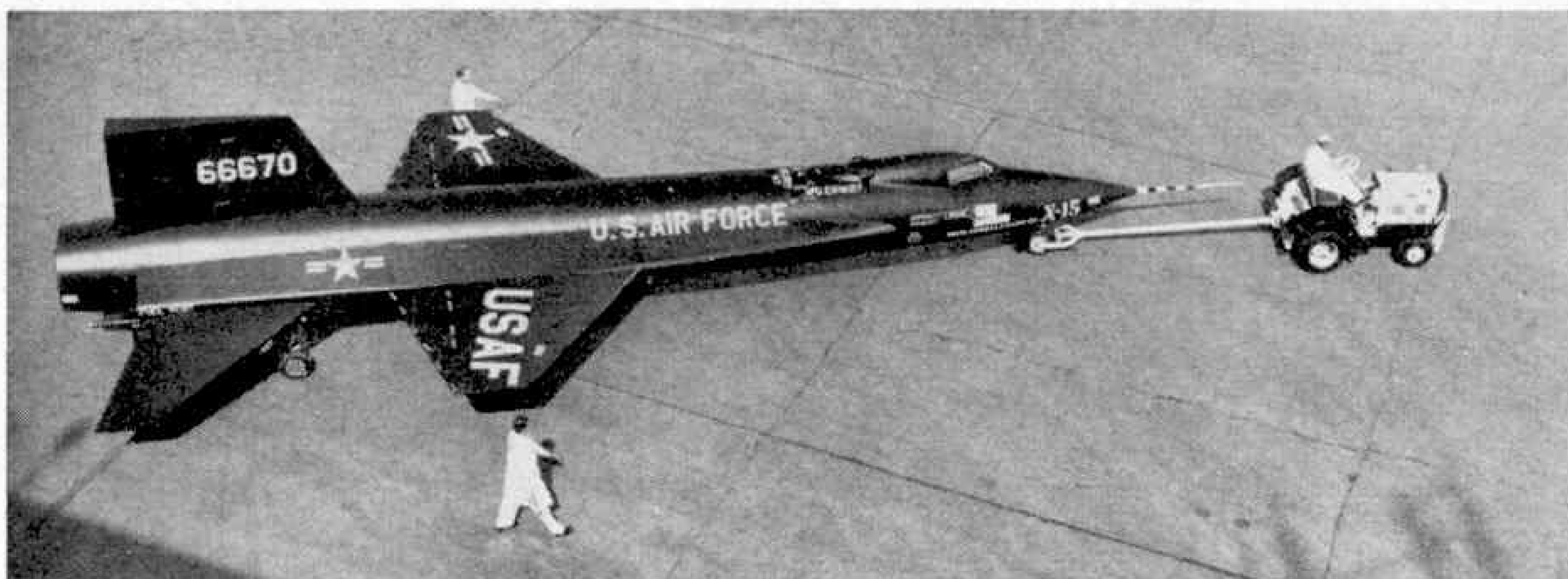
North American Aviation's X-15, the aeroplane designed to carry a man as far as 100 miles above the Earth and to fly at 3,600 miles per hour.
