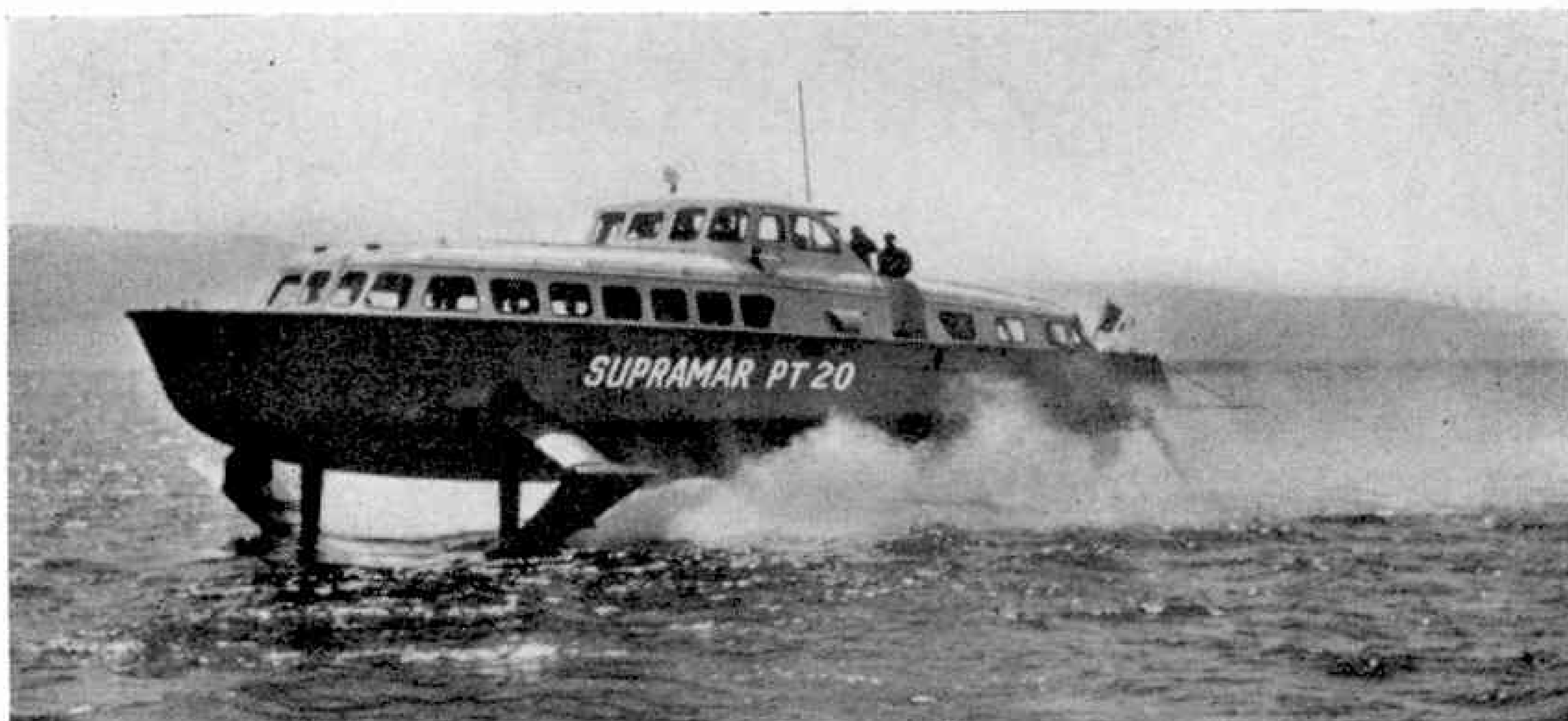
The Supramar hydrofoil vessel travelling fast with only its hydrofoils immersed in the water. Photograph Supramar A.G.
