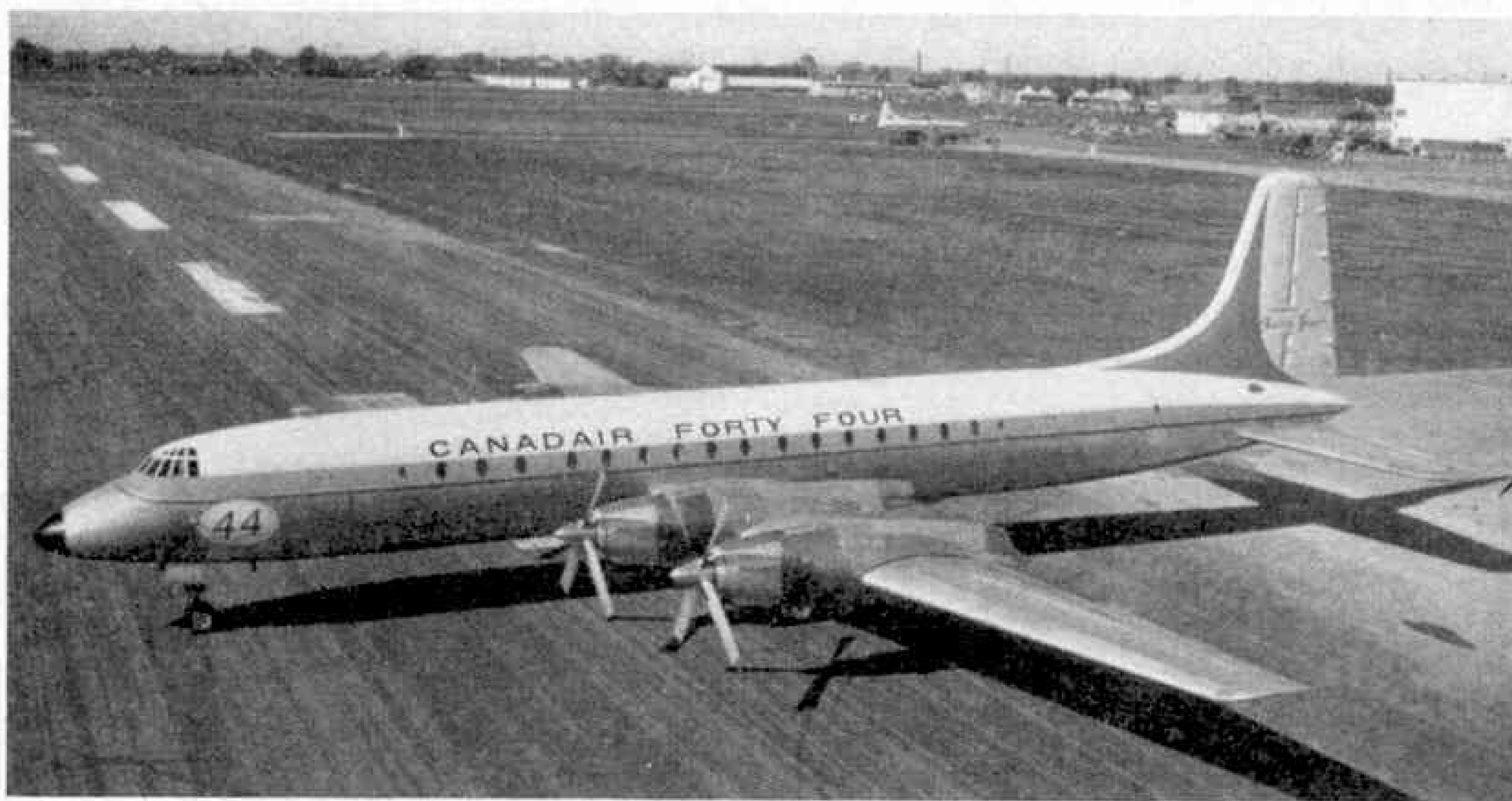
The Canadair Forty-Four long-range, four-engine, turboprop transport. It is the largest aircraft ever built in Canada.
