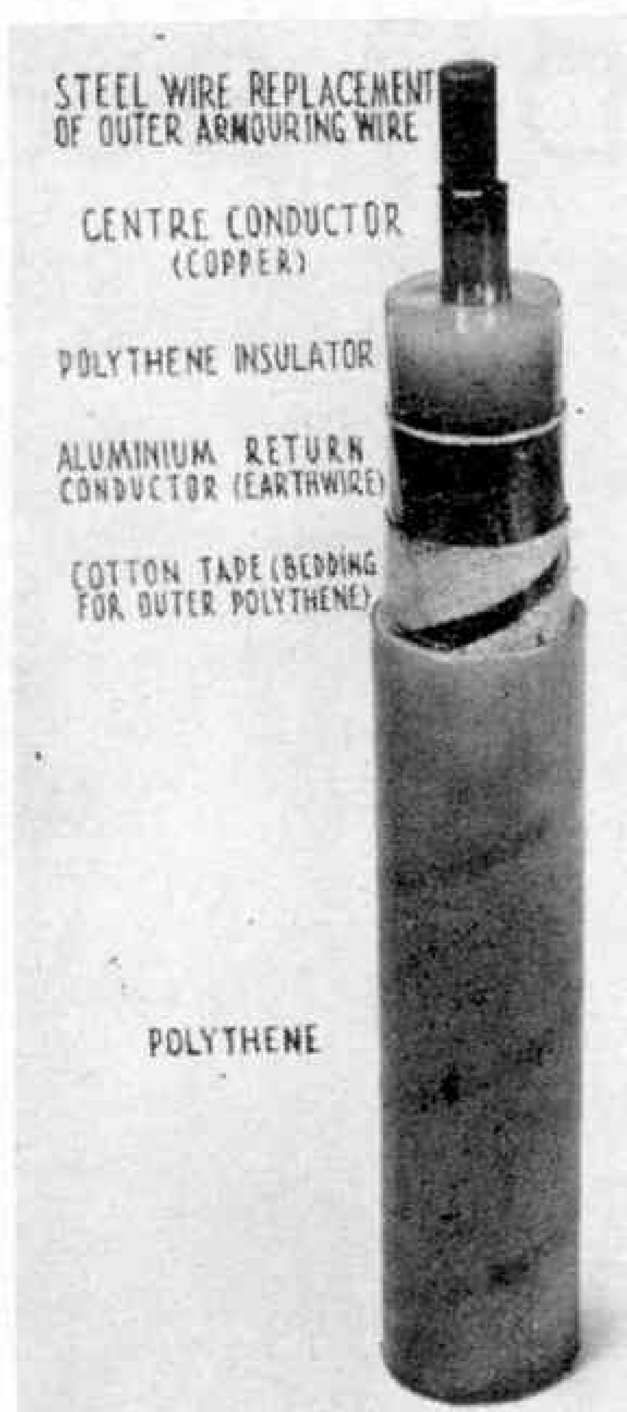
A section of light-weight unarmoured submarine cable. This photograph, and that on the preceding page, are reproduced by courtesy of Cable and Wireless Ltd.
