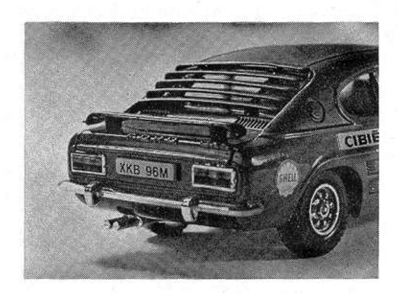
Above, a close-up of the rear of the Rally Capri, clearly showing the aerofoil stabilizer and rear louvres.
