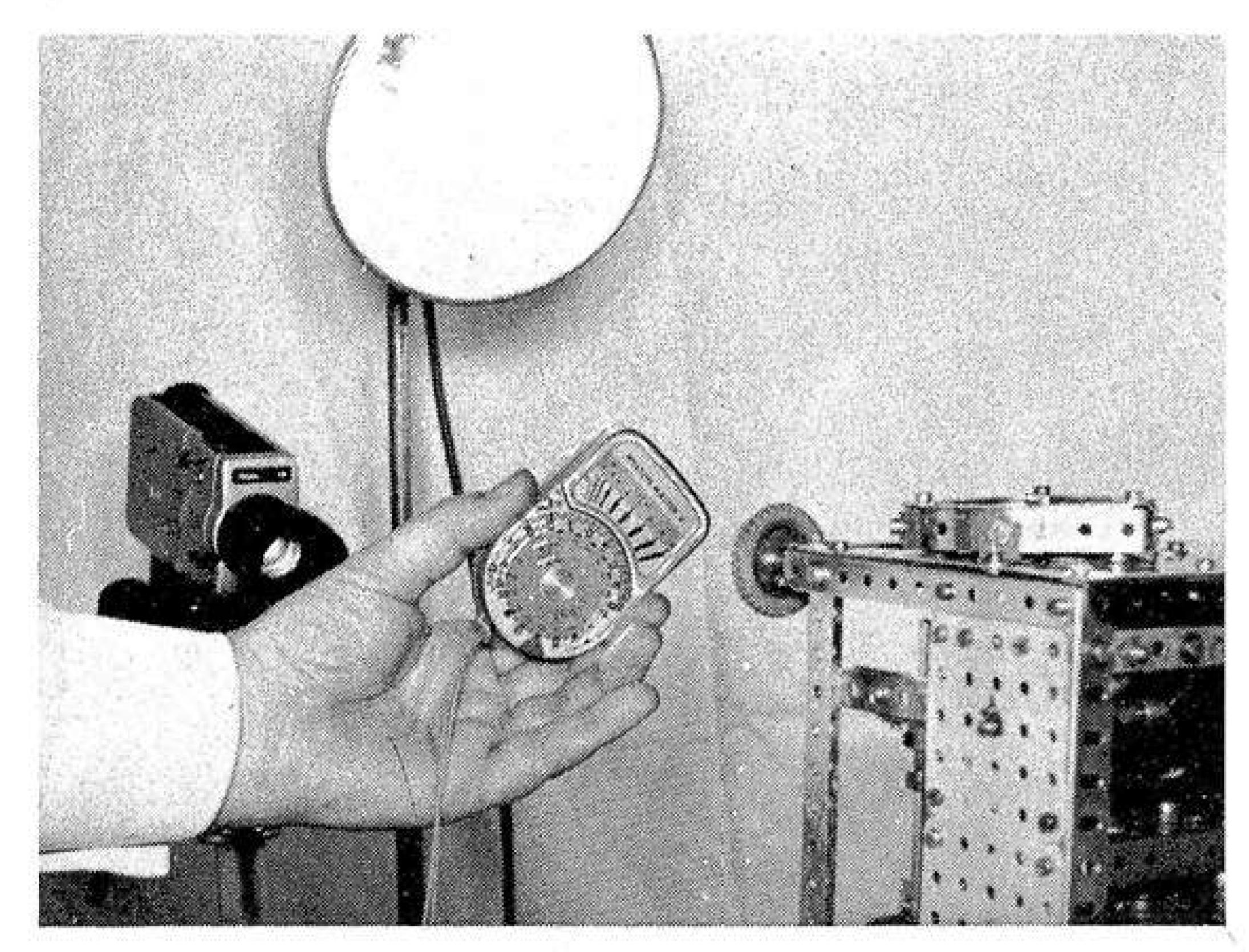
Fig.2. Using a separate exposure meter for calculating the correct exposure, showing the method of obtaining an "incident light reading".
