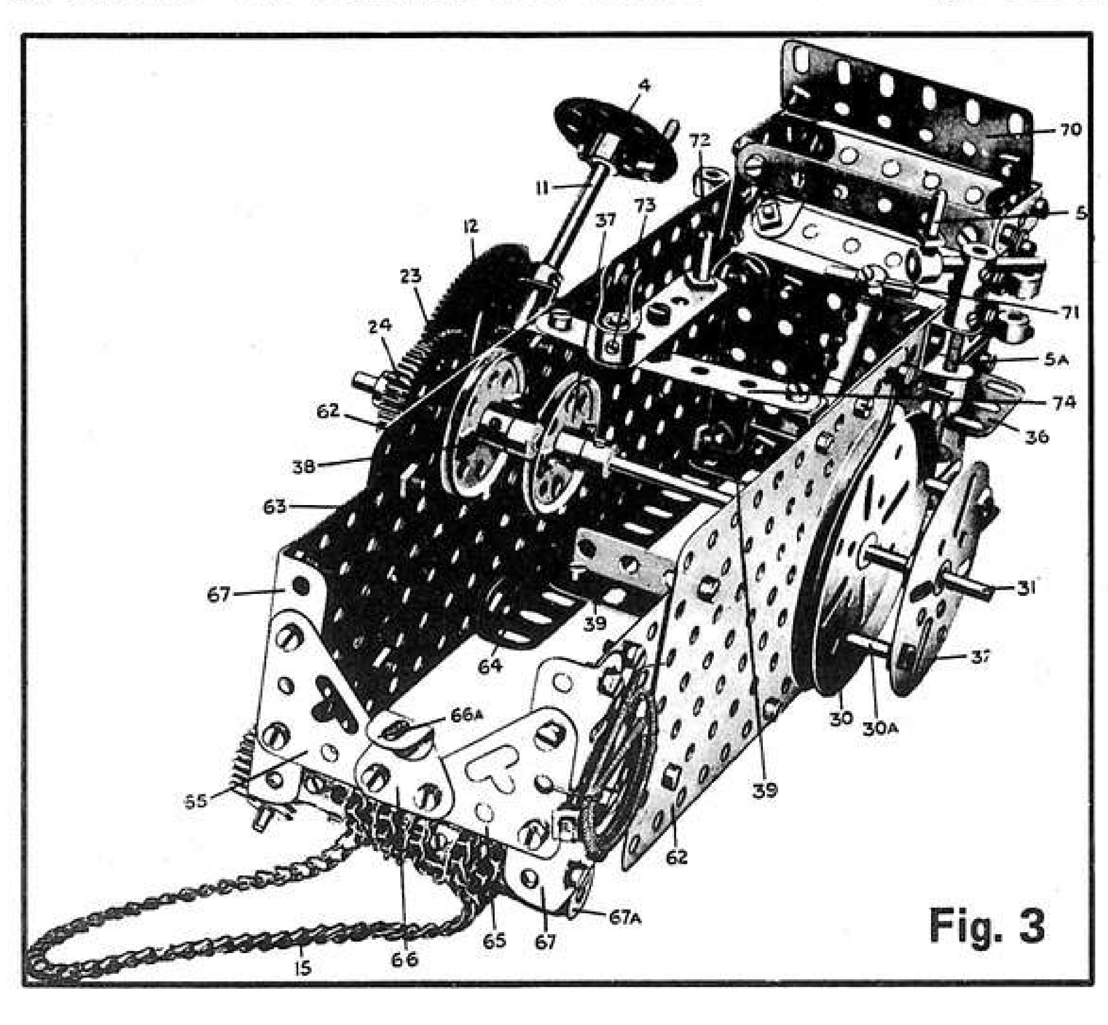
Fig. 1, opposite page, a general view of the circa 1930 S.M.L. No. 22 Meccano Traction Engine. Fig. 3, left, the main frame, showing control handles and rear axle complete with reinforced bearings (37). All illustrations in this feature are direct reproductions from the original Super Model Leaflet.
