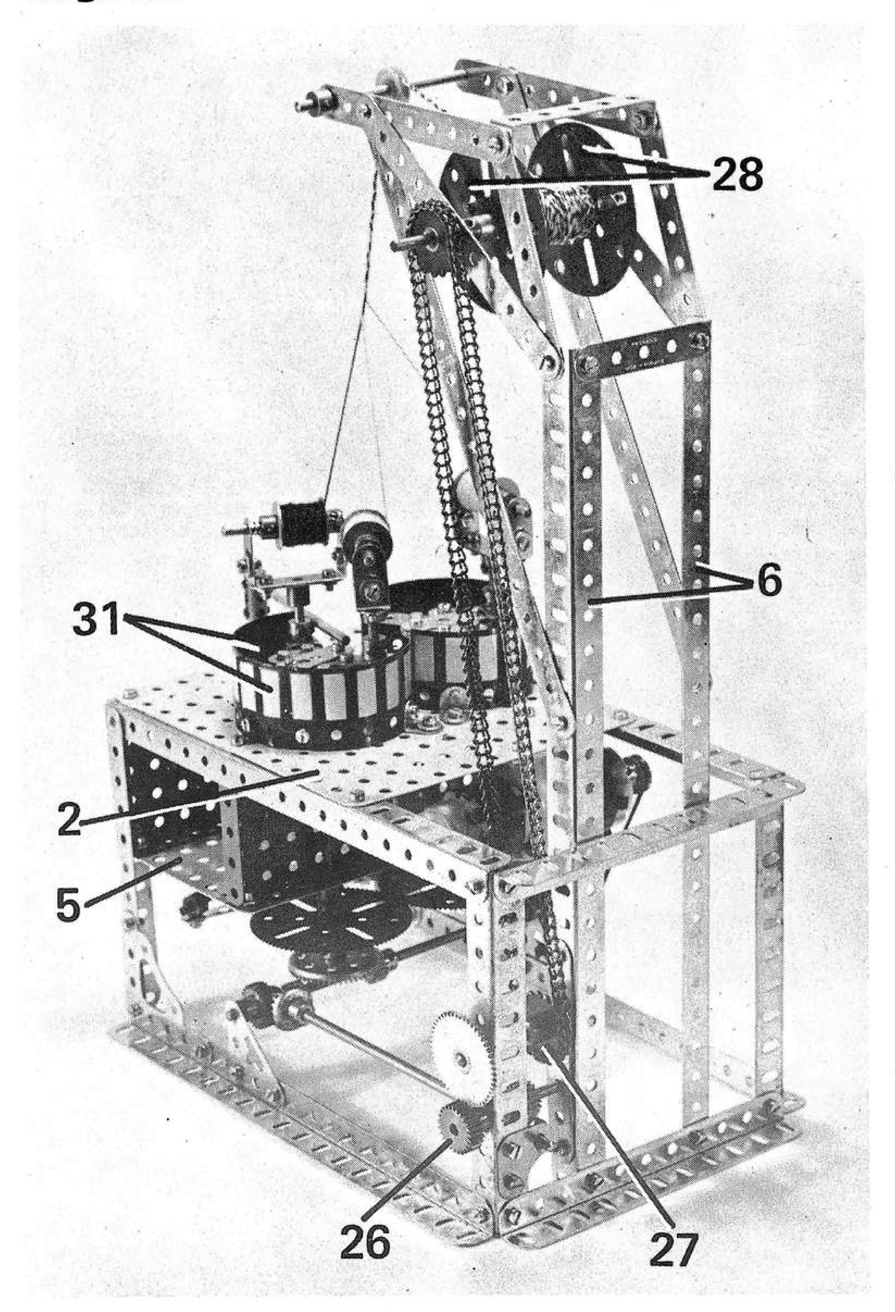
A rear view of the Plaiting Machine showing the drive to the cord take-up spool.
