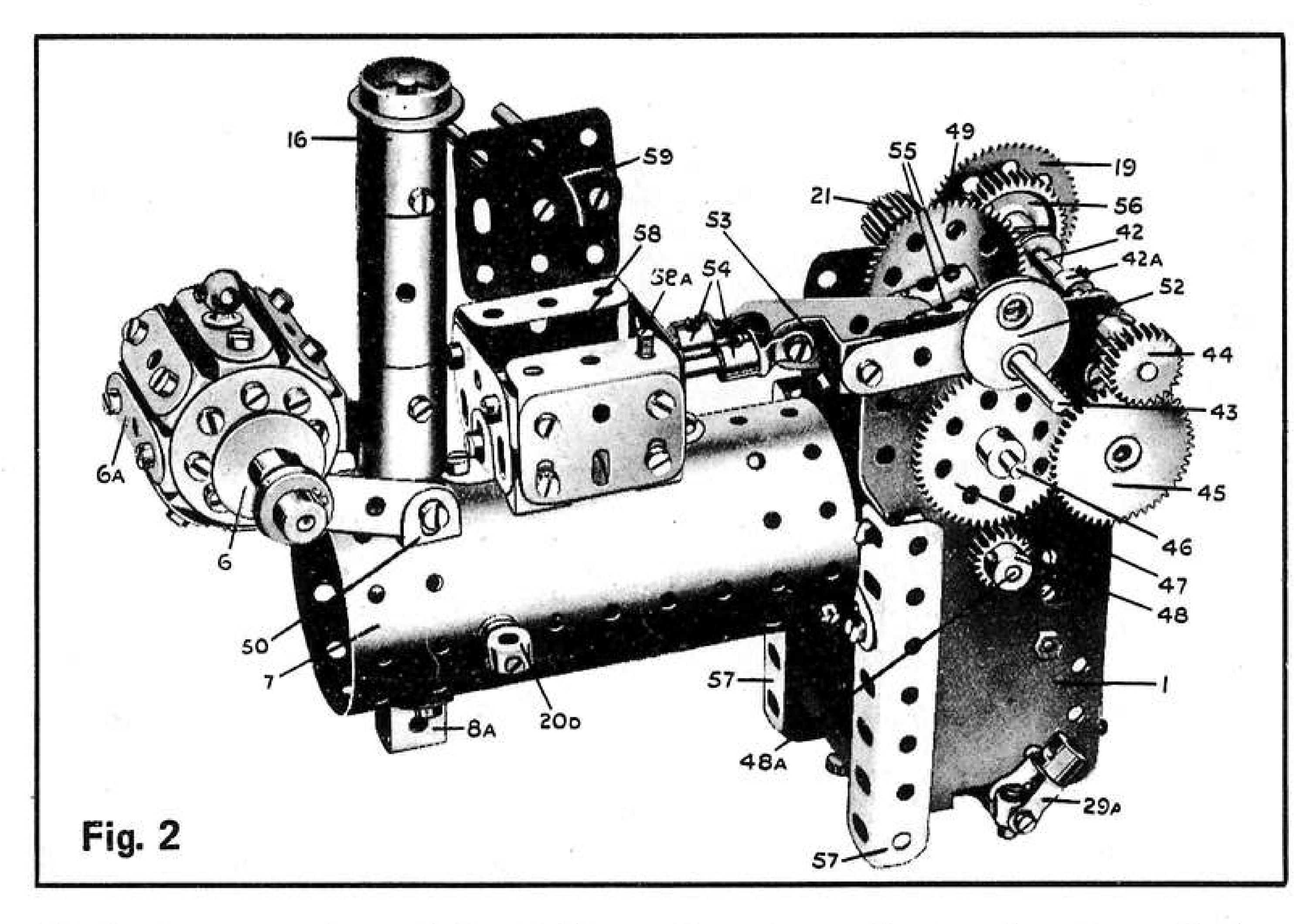
Fig. 2, above, a view of the boiler and motor unit, showing the cylinder block, dynamo, etc.
