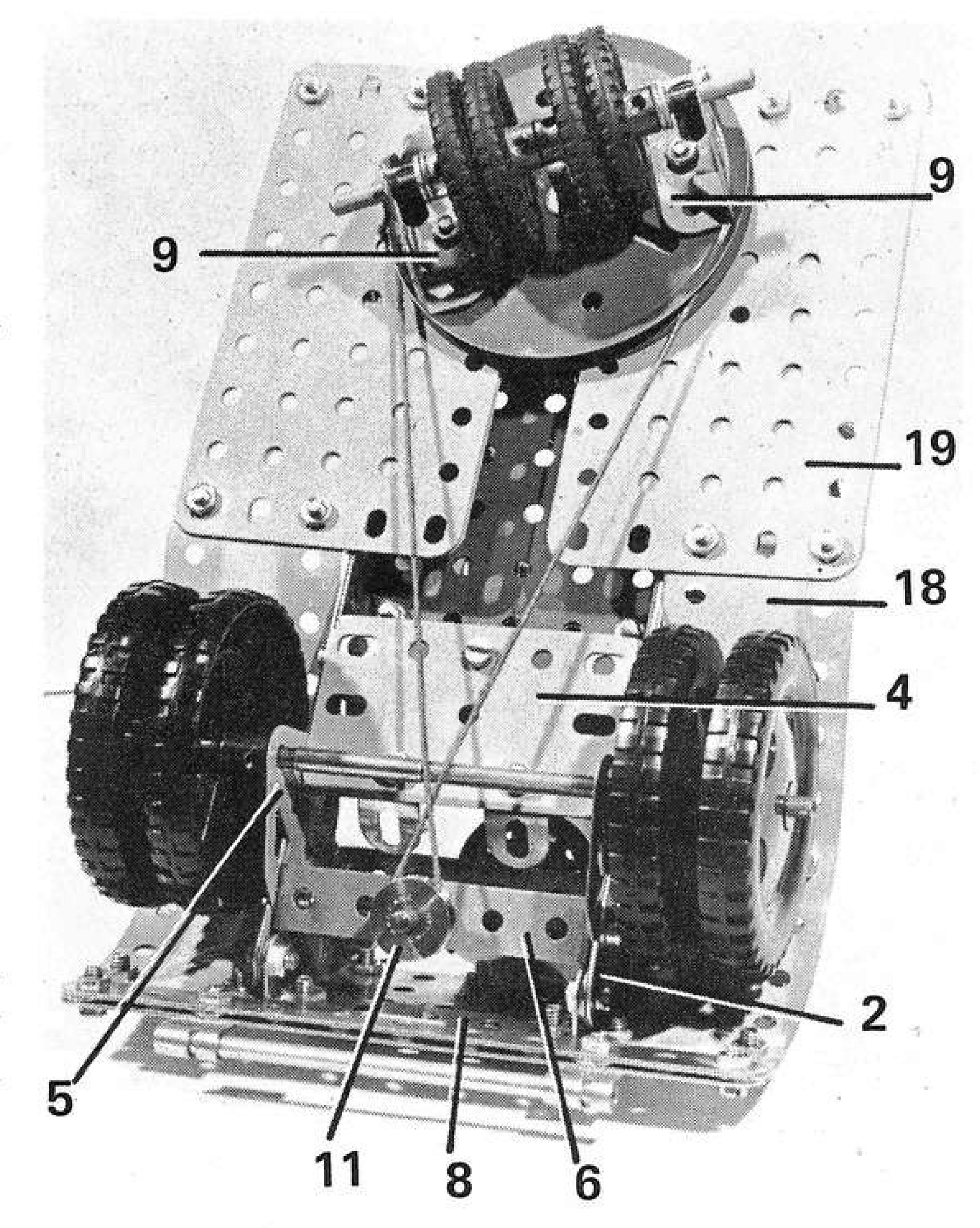
Right, an underside view of the Jumbo Crane showing the front axle assembly and the rear castor steering. Note the crossed-over steering cord.
