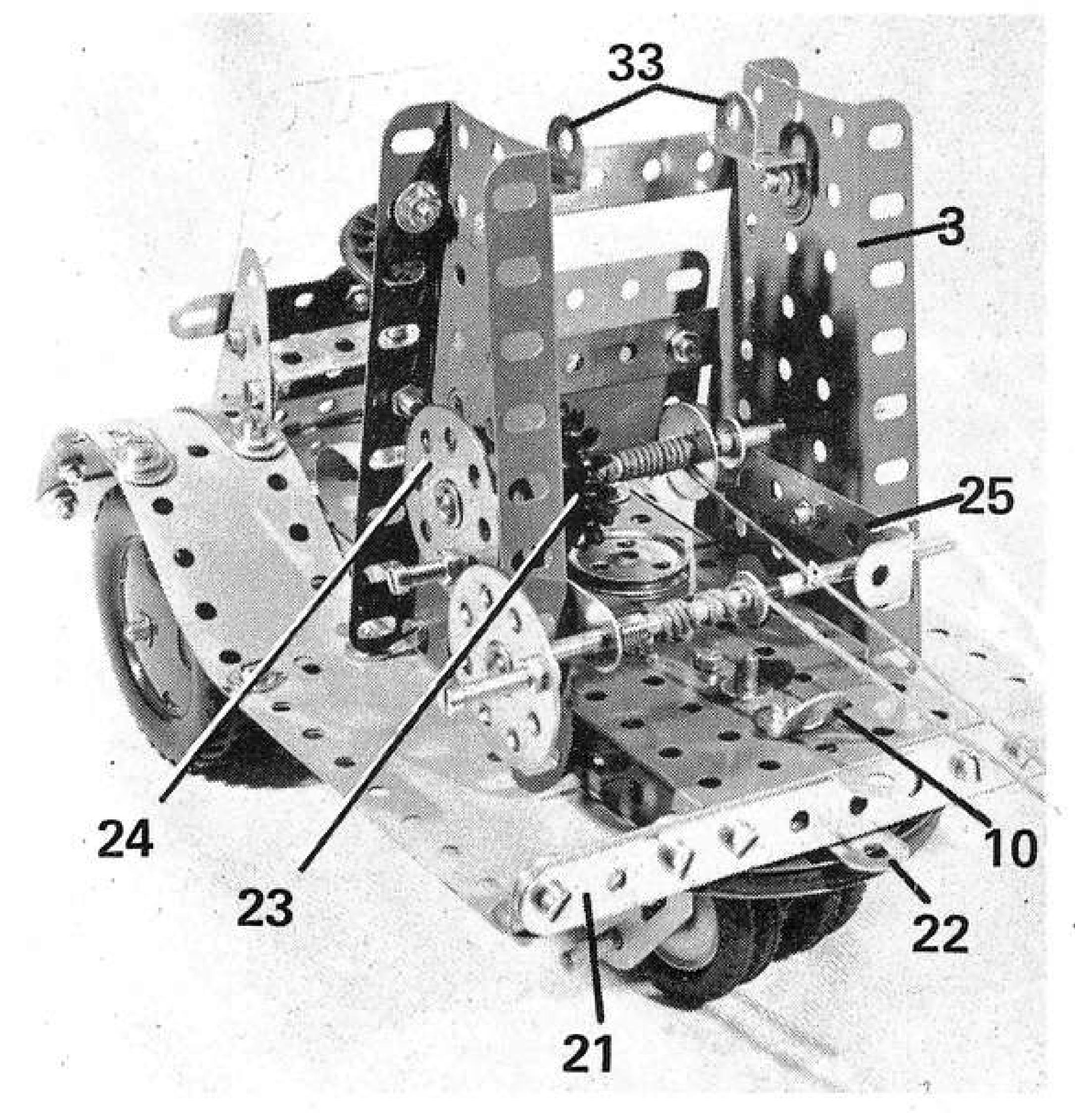
Jumbo Crane with the jib removed to show the hoisting and luffing winches. Both winch shafts must slide laterally their bearings. (Ignore the 1" Pulley shown lying on the main Flanged Plate this found its way in by mistake and was not spotted until after the photograph had been taken!).
