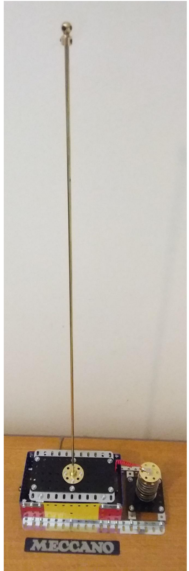
Fig 3. Brass rod antenna is 700mm long and has a part 136a Handrail Coupling on top.
