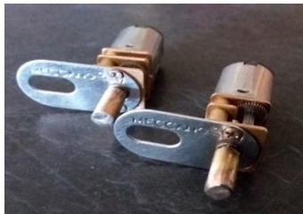
Fig.25 Motors mounted on Fishplates.
