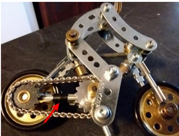
Fig.7 Spacers keep the chain tight
