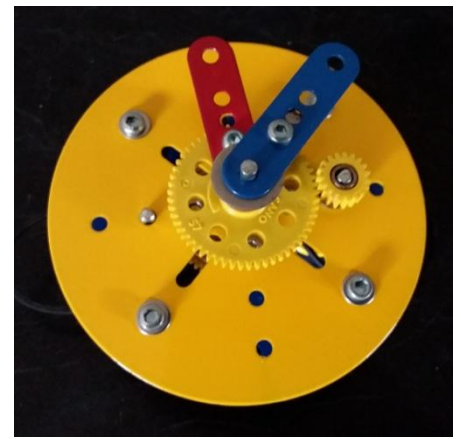
Fig.22 Red hand mounted on 57t Gear. Blue hand mounted on a Crank.
