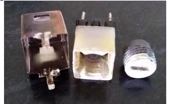
Fig 6. The thread is stripped.
