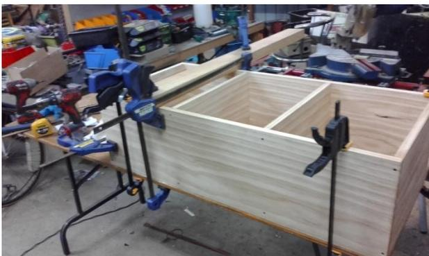
Before the PVA glue dries you can tap the shelves to get them perfectly square and flush then it's just a matter of screwing them in. I used 75mm square head screws but nails would do. I doubt the shelves would hold the heavy cases laden with parts unless you used screws or nails.
