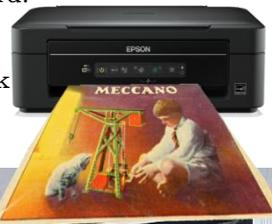
**Step 16.** Labels are photocopied from good originals using a laser printer. This gives a good image as well as being shiny and durable. Inkjet printing just doesn't cut it! I have eight pretty good originals so I could vary the labels when I make the repro boxes. Nothing worse than the photo shopped cartoon look that some do to make an original label look "new".
