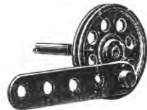
N —Crank formed with 1\frac{1}{2} " pulley wheel and strip, lock-nutted.
