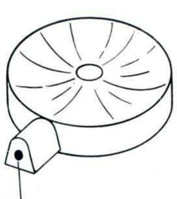
Hole 4mm diam. to be drilled in position shown above
