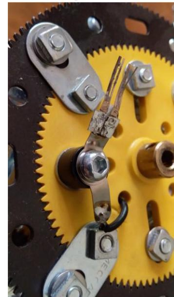
colour and excitement to the ride I have added strips of LEDs in the centre. This necessitated the use of a commutator and wiper. I think the Elektrikit wipers are less than adequate as they have a dimple that gradually wears through the commutator so I have fashioned my own using wipers salvaged from old motors. See close up at left.
