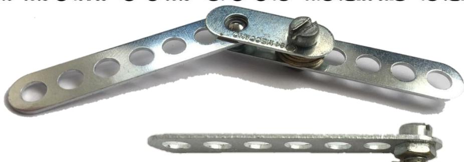
No slop pivot joint based on an original design by Bert Halliday. The 3/16" ball sits between the 7 hole Narrow Strips and the 2 hole Narrow Strip locks it into place. Richard Payn.
