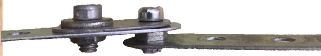
Another easy way of doing a play-free joint. Make the hole smaller by clamping a fishplate over the hole then slide it do the bolt just goes through. Then locknut a strip below. Richard Payn.
