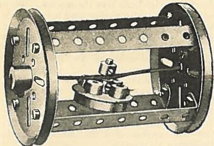
The weight illustrated comprises a Flanged Wheel carrying four Collars, the set-screws of which grip the shank of bolts passed through the Flanged Wheel.
