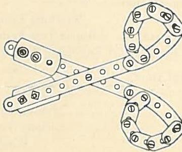
screwed to the bolts are used as a pivot and these are lock-nutted together by tightening one against the other, which prevents them from becoming loose. Enough play is allowed in the bolt to permit of easy movement of the strips. The following parts are required to build the scissors: 2 of No. 2, 2 of No. 90, 12 of No. 10, 4 of No. 38, 20 of No. 37, and 2 razor blades.
