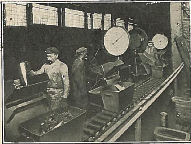
*Weighing of metal previous to melting*
