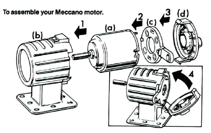
Position motor (a) in motor housing (b) with end contacts at top and bottom (see inset). Locate the switch lever (c) (smooth side outwards) over the motor end contacts.
