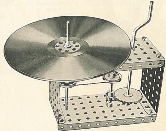
This is a model to show that white light is made up of the three primary colours—red, yellow, blue. Sectors of these three colours are mounted or painted on the disc, which if then quickly rotated, shows as white.
