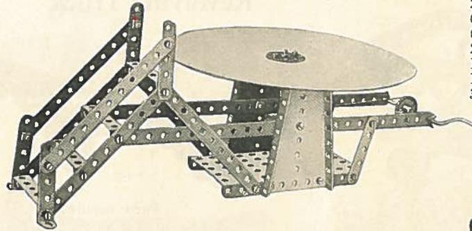
The driving mechanism and construction of the framework of this model are clearly brought out in Fig. 206A. Cut out a circular piece of cardboard, 8" in diameter, and in the centre of the disc fix a bush wheel by nuts and bolts. The eye of the bush wheel is then threaded over the top of a vertical spindle, and secured by its set-screw.
