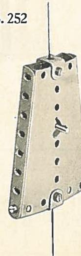
When the cord is held vertically the magic sector plates will fall or stop at the bidding of the owner. If the cord is held without tension the plates will fall, but the instant the cord is tightened they will stop dead. The cord is wrapped once around the rod which passes through the centre holes of the sector plates.
