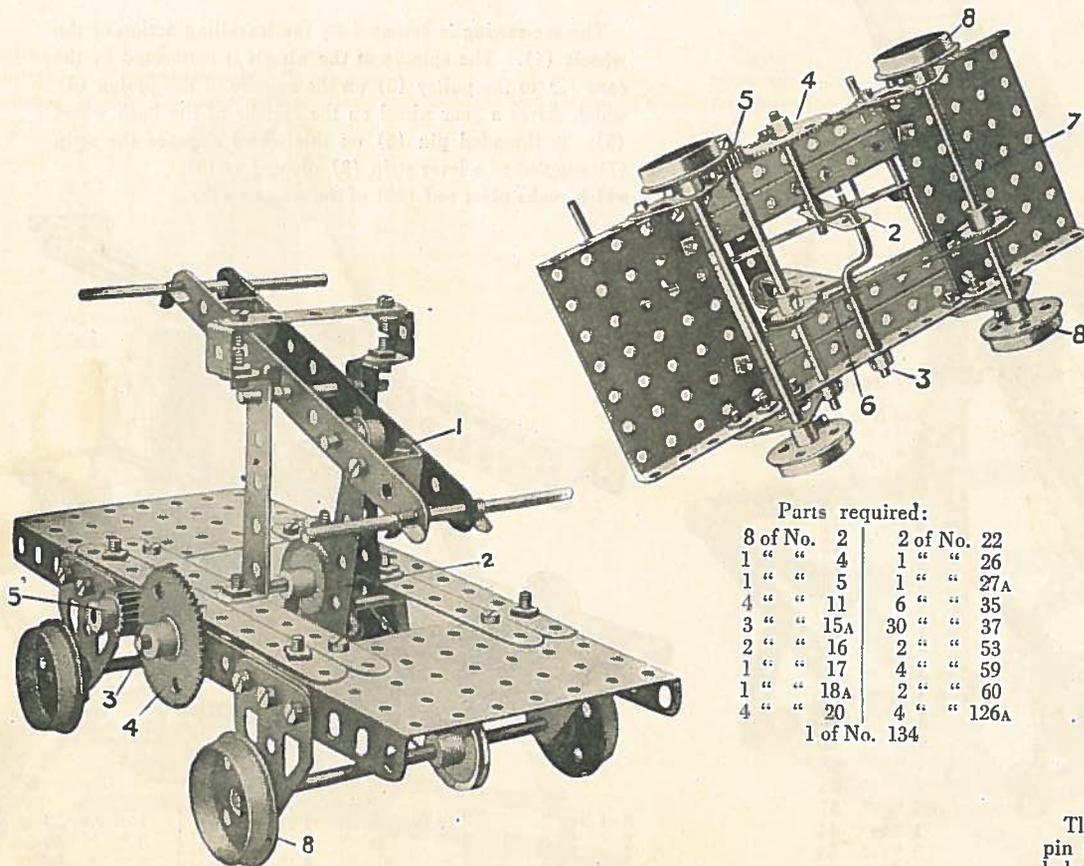
The car is caused to travel by working the rocking lever (1) which is connected by a strip (2) to a crank shaft (3) and a gear wheel (4) meshing with a pinion (5) on a rod coupled by a cord (6) to an axle rod (7) of the travelling wheels (8).
