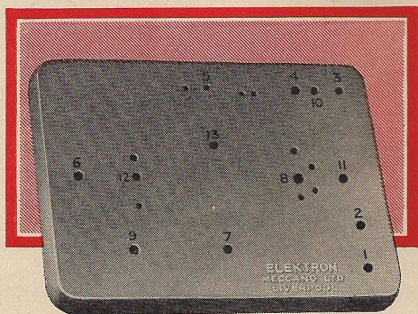
Fig. 22. The Elektron Universal Base. Terminals and other parts fit the large numbered holes, and connecting wires only are passed through the smaller openings.
