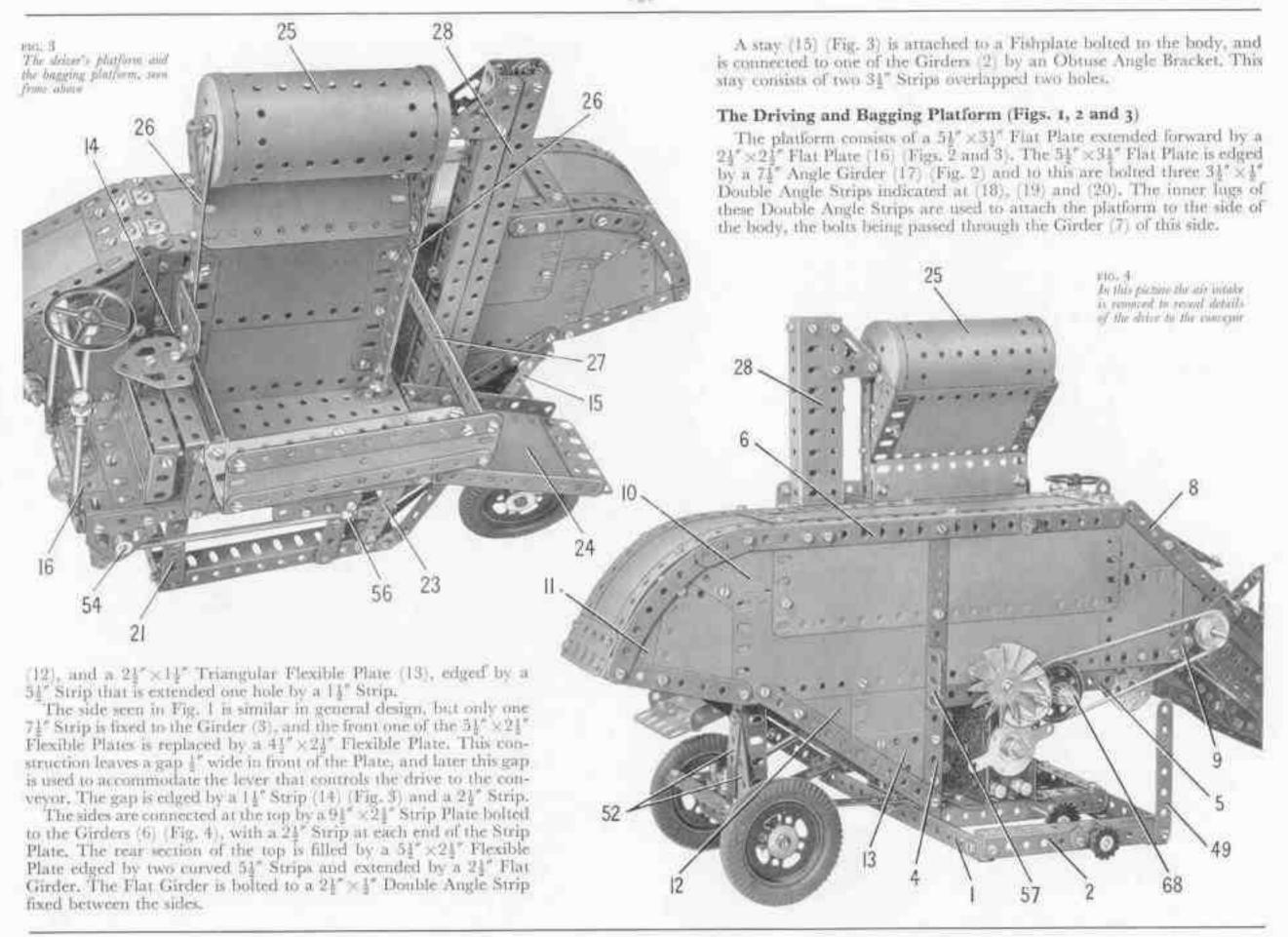
A built-up strip (21) (Fig. 3), made from two 2" Strips overlapped two holes, is bolted to one of the Girders (2) (Fig. 2) and is connected to Double Angle Strip (19) by an Angle Bracket, A 3" Angle Girder (22) (Fig. 10) is fixed to one of the Girders (1) and is attached to the Double Angle Strip (19) by a 4" Corner Angle Bracket (see Fig. 10). A 34" Strip (23) is secured to the Girder (17) and is connected to one of the Girders (2) by an Obtuse Angle Bracket.
